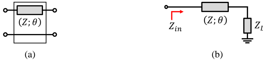
Figure B.2 – (a) Transmission Line representation as a two-port network, (b) Transmission line terminated in a load Z_L
