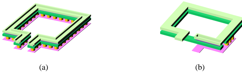
Figure 4.26 – Custom inductor with (a) High quality factor, (b) High compactness.
