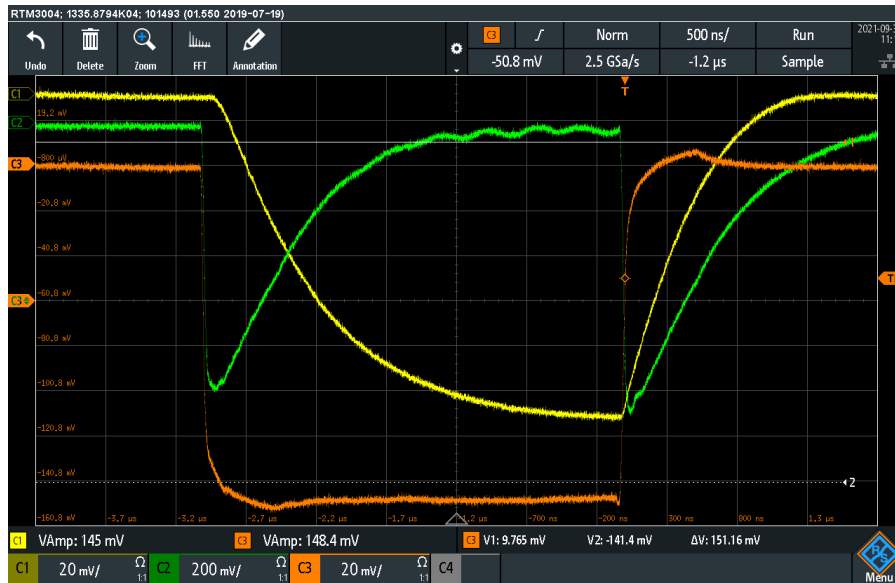
Figure 3.6: RF power signals measured by an oscilloscope ( P_{ic} in brown, P_{rc} in green and P_{bc} , which is the visualised power inside the cavity, in yellow).
