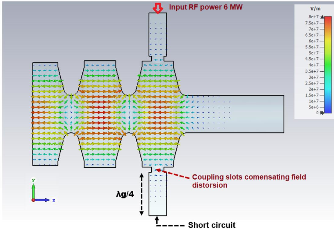
Figure 2.25: Electric field (accelerating mode  $TM_{010-\pi}$ ) distribution in the ThomX photoinjector with a input RF power of 6 MW simulated using CST Studio Suite®.
