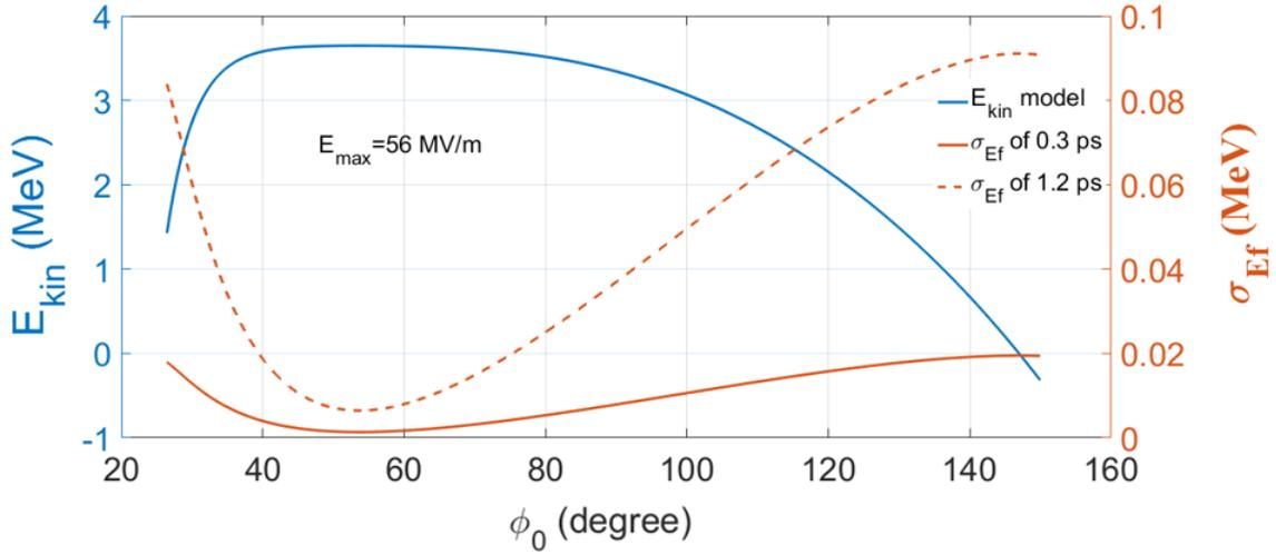
Figure 3.29: The kinetic electron energy  $E_{\text{kin}}$  simulated from Eq.3.9 and the energy spread  $\sigma_{E_f}$  simulated from Eq.3.16 for 2 bunches (0.3 ps and 1.2 ps) as a function of the RF phase  $\phi_0$  at the photoinjector exit ( $z=0.125$  m) for  $E_{\text{max}}=56$  MV/m (to simplify,  $\sigma_{E_i}$  and  $\sigma_{E_{t_i}}$  are assumed to be 0 keV and 0 MeV.ps respectively).
