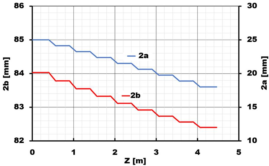
Figure 2.36: Cell iris diameter (2a) and cell inner diameter (2b) as a function of z along the structure.
