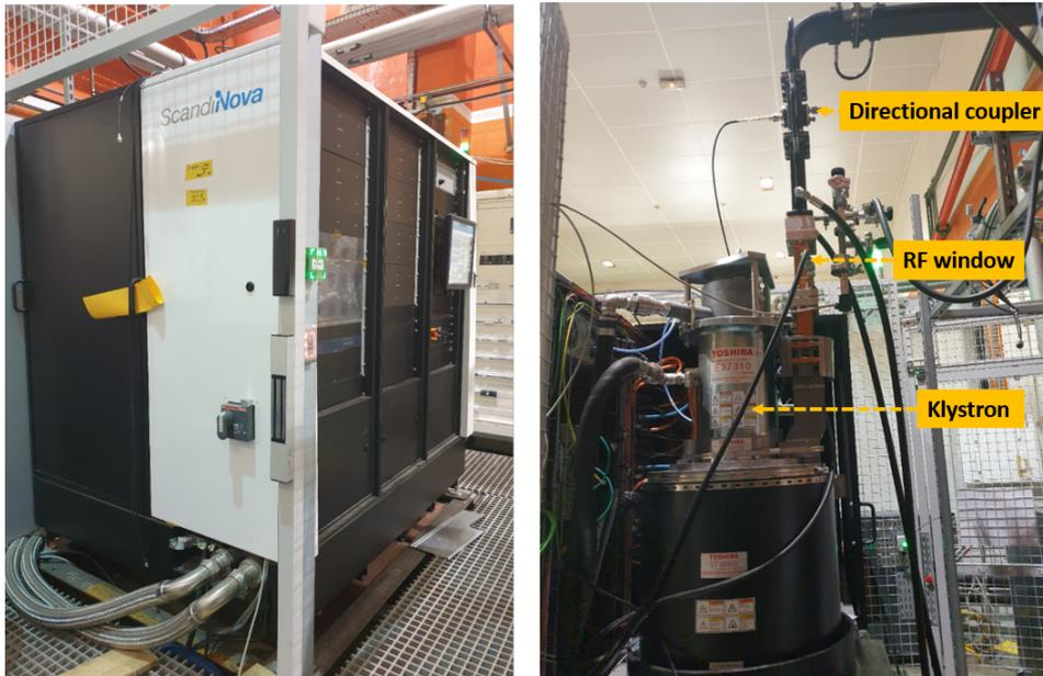
Figure 2.9: Installation of the ThomX RF source (ScandiNova modulator K2-2 & TOSHIBA Klystron E 37310).
