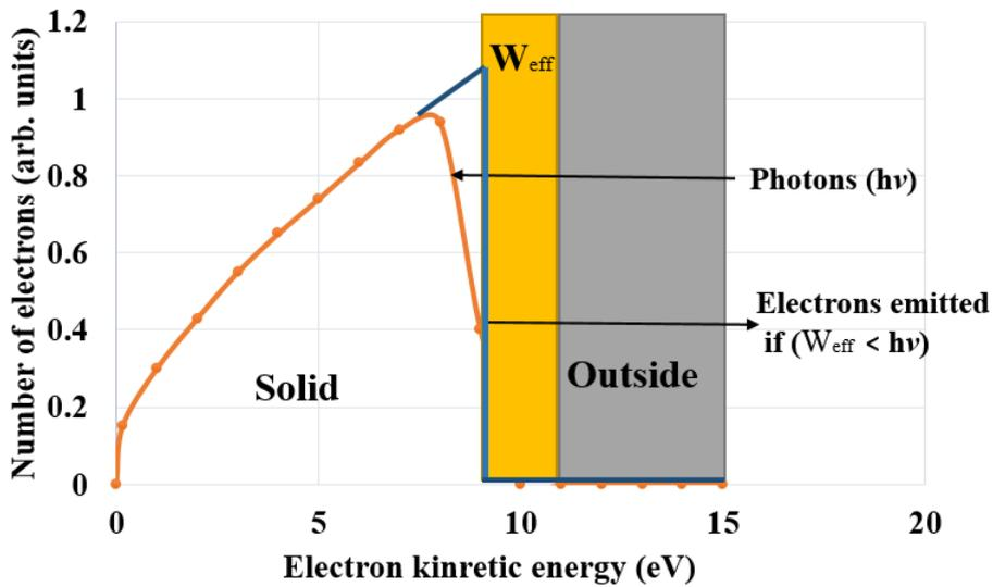
Figure 3.11: The basic physical principle of the photoelectric emission.  $W_{\text{eff}}$  is the work function of the material and  $h\nu$  is the photon energy, with  $\nu$  the photon frequency and the Planck constant  $h = 6.626 \times 10^{-34}$  J.s. Blue curve: 0 K; Orange curve: 2000 K [53].
