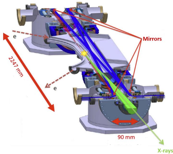
Figure 1.6: Layout of the ThomX Fabry Perot cavity [12].
