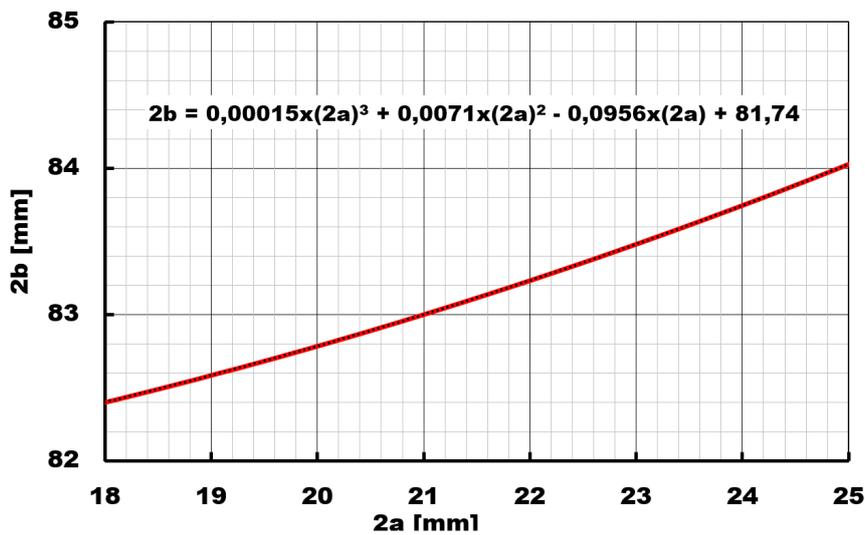
Figure 2.37: Inner cell diameter (2b) as a function of iris cell diameter (2a) at 2998.55 MHz (in vacuum at 30 °C).
