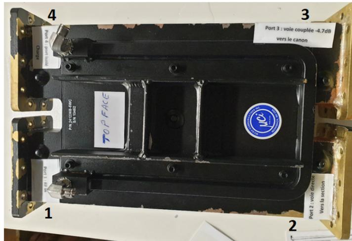
Figure 2.12: Identification of the power divider inputs and outputs.
