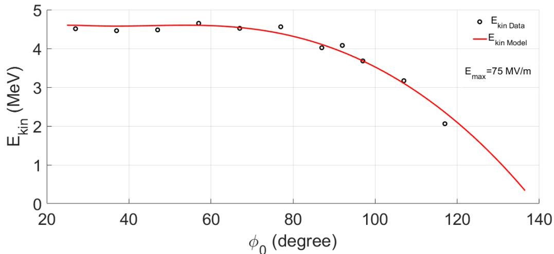
Figure 3.20: The experimental and analytical electron kinetic energy  $E_{kin}$  at the exit of the ThomX gun as a function of the RF phase of the photoinjector  $\phi_0$  at  $E_{max}=75$  MV/m.
