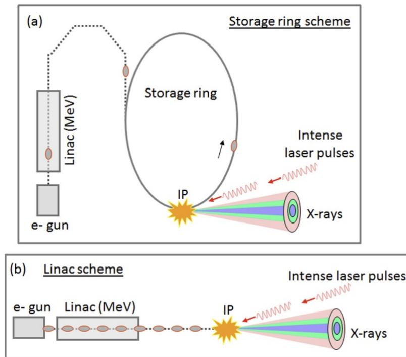
Figure 1.4: Schematic diagrams of compact Compton based X-ray sources; (a) a storage ring scheme, (b) a linac scheme [18].
