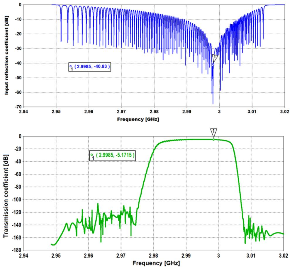
Figure 4.7: Input reflection coefficient (upper plot), transmission coefficient “insertion loss” (lower plot) versus frequency of the whole structure.
