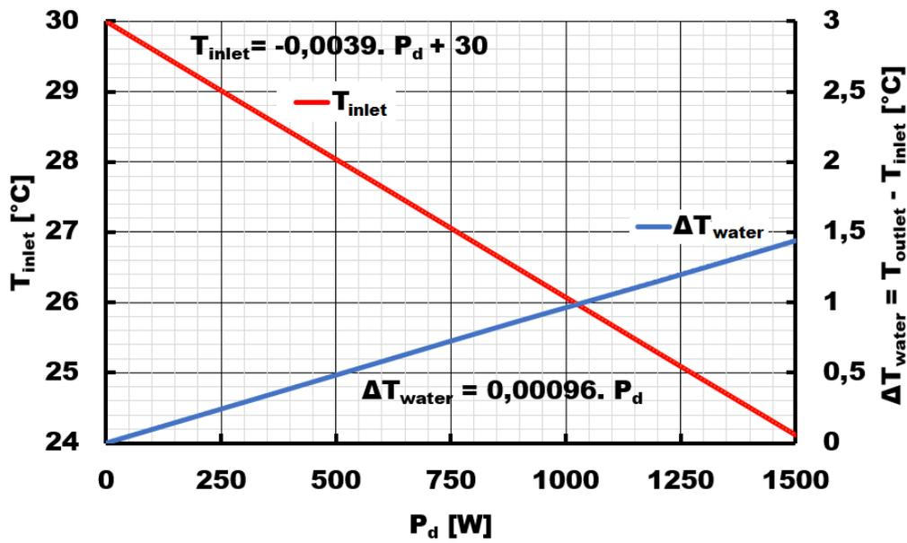
Figure 2.45: Water inlet and outlet temperatures as a function of the dissipated power into the RF gun with a nominal water flow rate of 15 l/min ( $T_{set} = T_{structure}=30^{\circ}C$ ).
