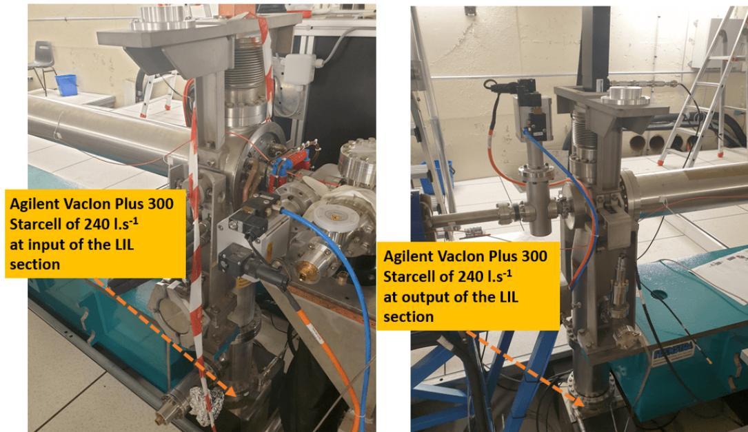
Figure 2.48: Ion pumps installed on the LIL structure.
