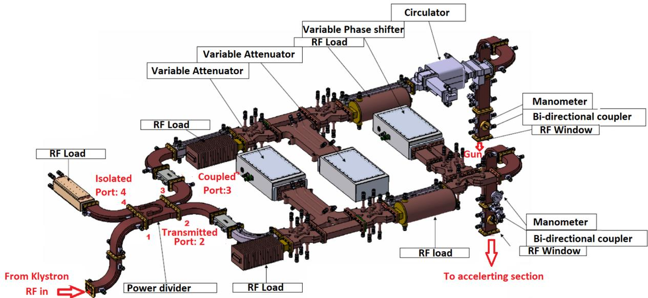
Figure 2.10: 3D drawing of the ThomX Power distribution network.
