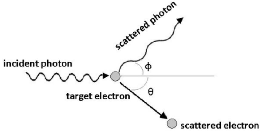
Figure 1.1: Schematic diagram of the Compton scattering process [15].
