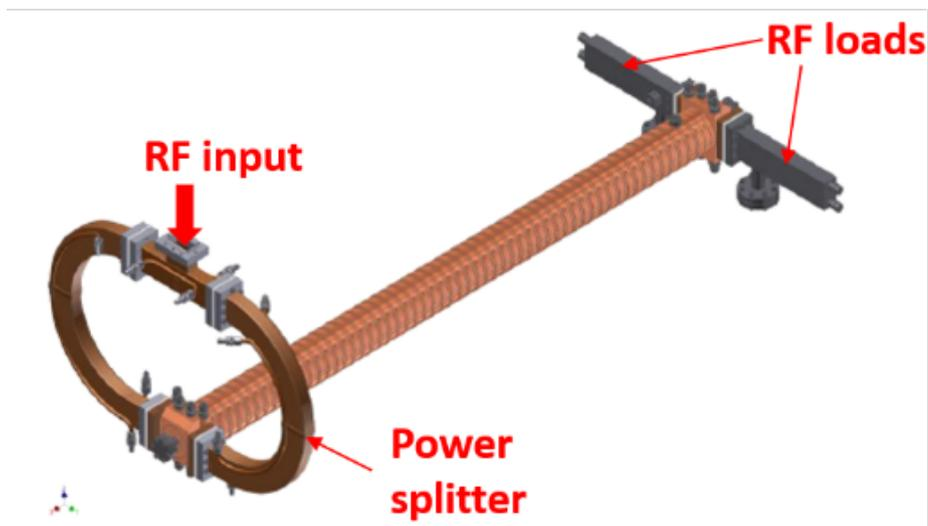
Figure 4.2: Mechanical design of the RI S-band structure.
