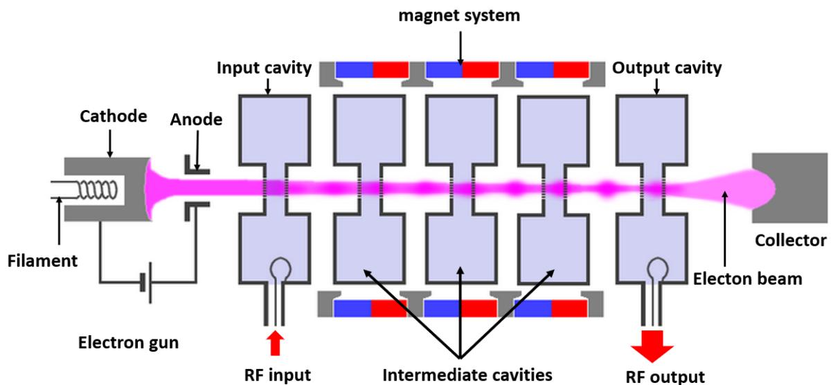
Figure 2.2: Diagram of a klystron tube amplifier.
