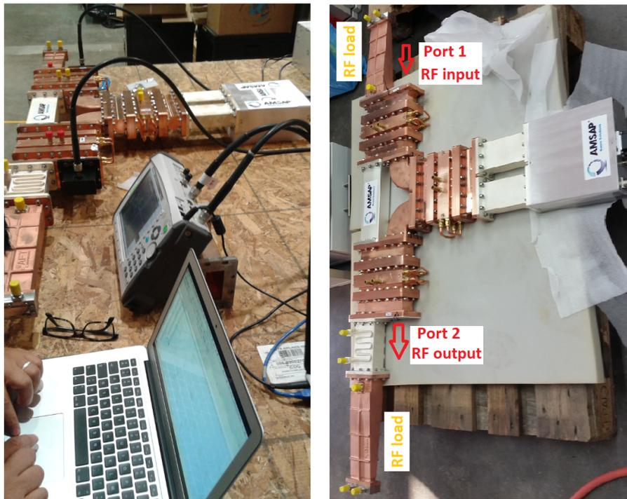
Figure 2.17: ThomX attenuator under test.
