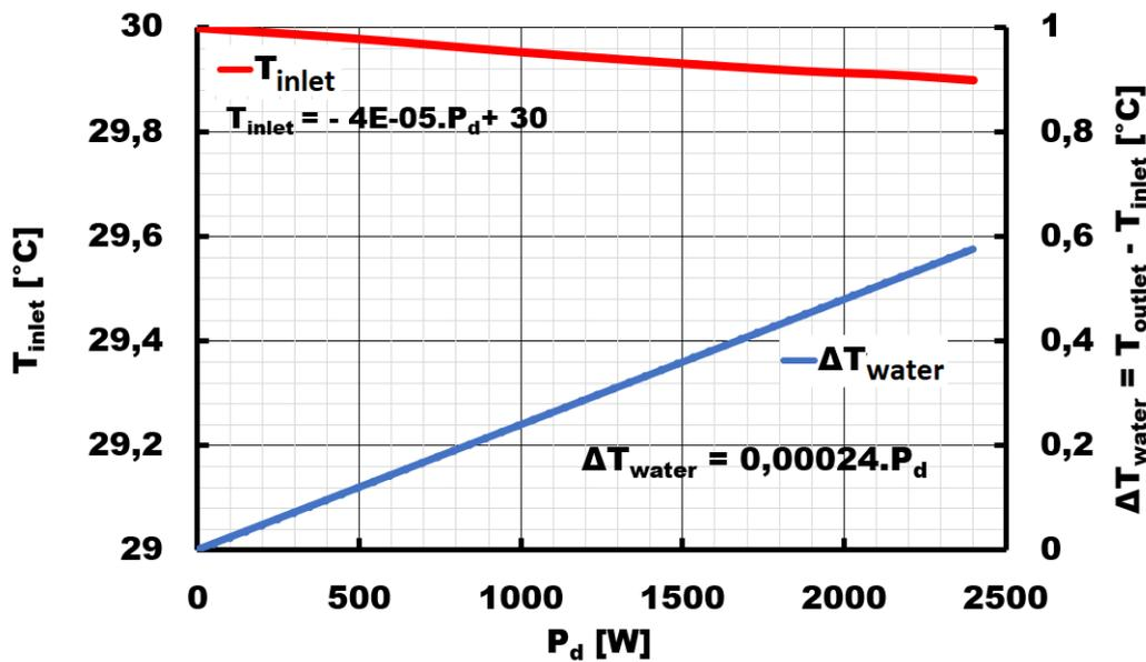
Figure 2.46: Water inlet and outlet temperatures as a function of the dissipated power into the LIL structure with a nominal water flow rate of 60 l/min ( $T_{set} = T_{structure}=30^{\circ}C$ ).
