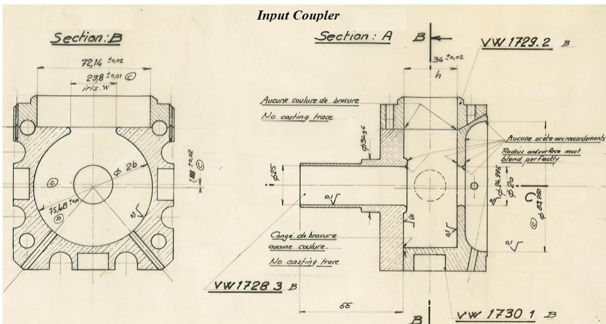
Figure A.2: Section drawings of the LIL input coupler.
