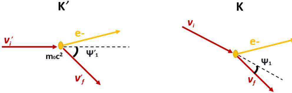
Figure 1.3: In the electron frame of reference, the photon is scattered with an angle  $\Psi_1'$  according to the conservation of energy and momentum (left). In the frame of reference K, the scattering angle is  $\Psi_1$  (right) [14].
