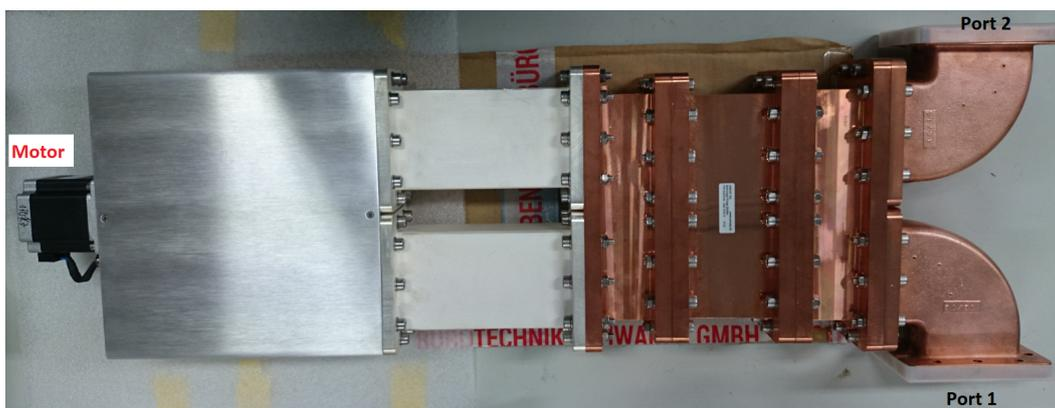
Figure 2.14: Picture of ThomX motorised phase shifter (S/N 170117).
