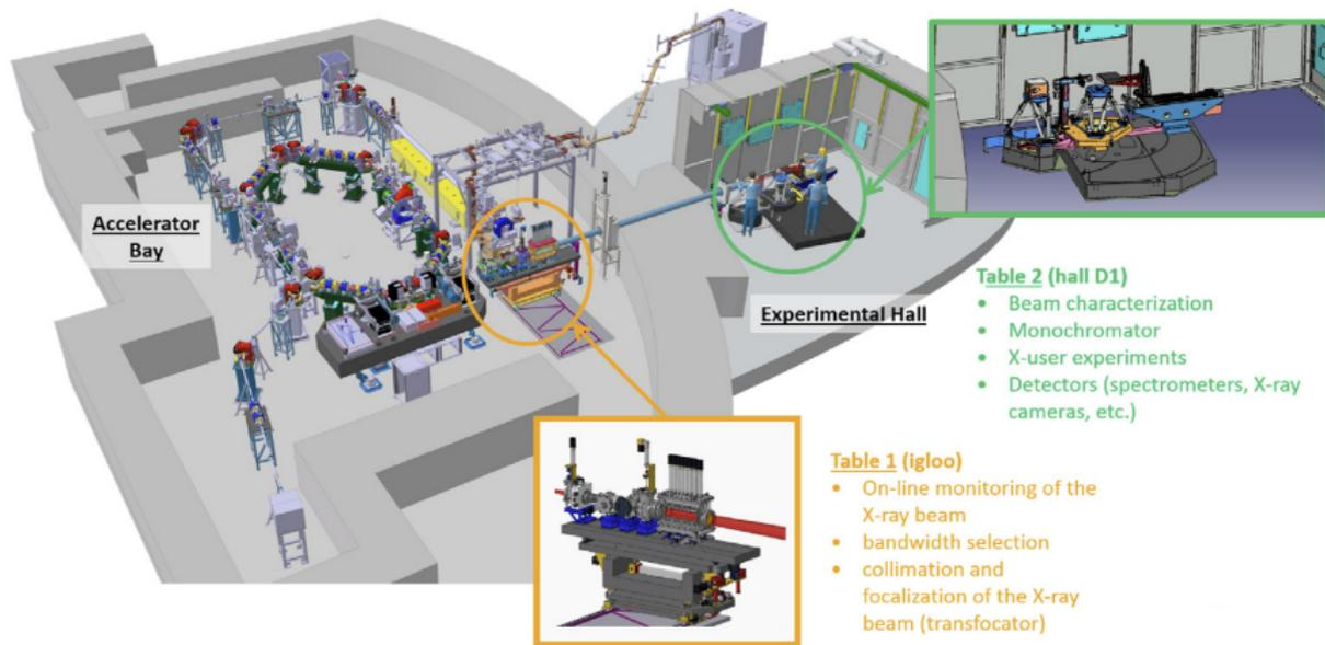
Figure 1.7: Layout of the X-ray line in ThomX [13].
