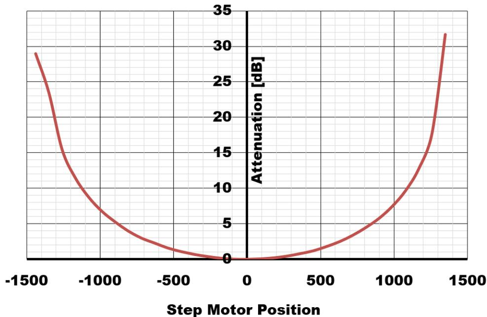
Figure 2.18: Attenuation measurement of the ThomX attenuators at 2998.5 MHz.
