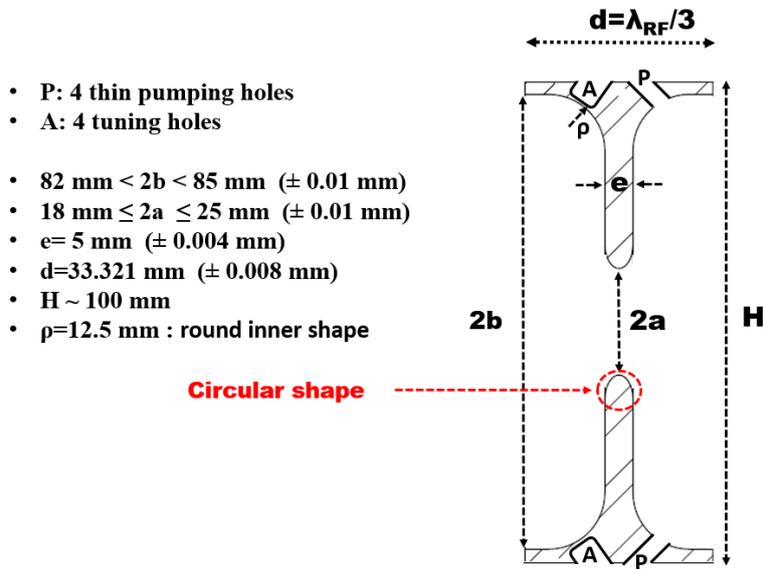
Figure 2.34: Mechanical aspects of a LIL cell unit.
