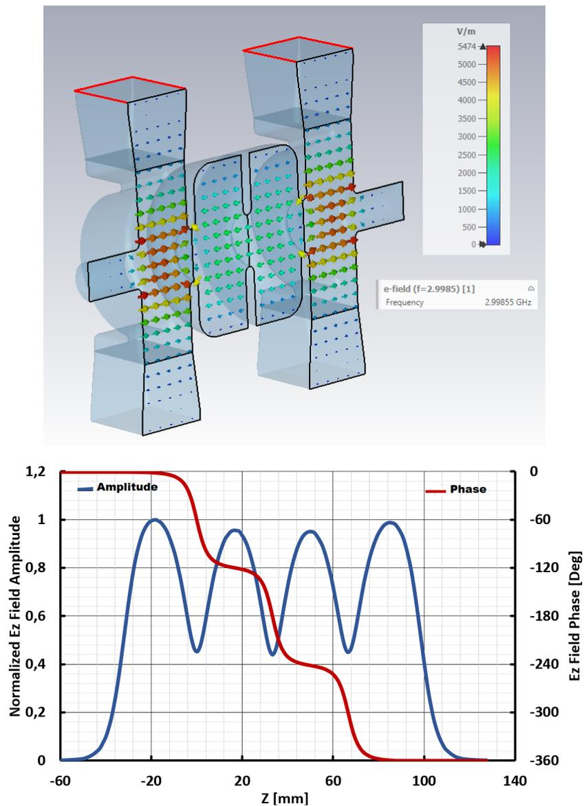
Figure 4.4: Reduced copper cavity model: Longitudinal electric field  $E_z$  (TM<sub>010-2π/3</sub>) distribution (upper). Normalised  $E_z$  field amplitude and phase ( $E_z$ ) on axis at working frequency 2998.55 MHz (30°C in vacuum) (lower).
