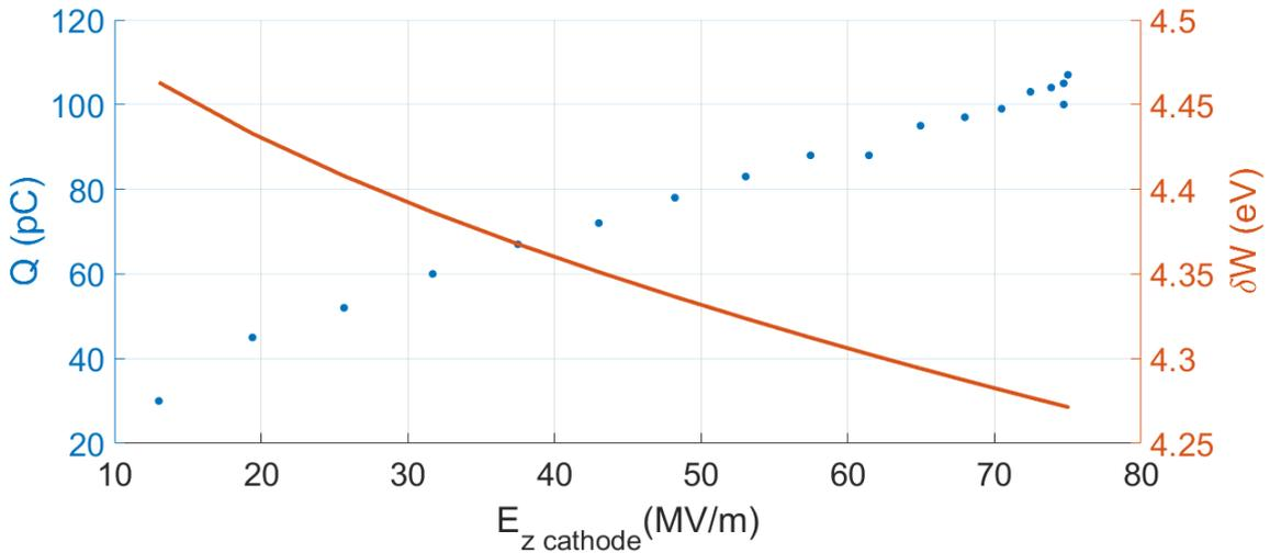
Figure 3.14: The measured charge  $Q$  (blue) and the lowering of the work function  $\delta W$  (orange) as a function of the accelerating field on the photocathode  $E_z$ .
