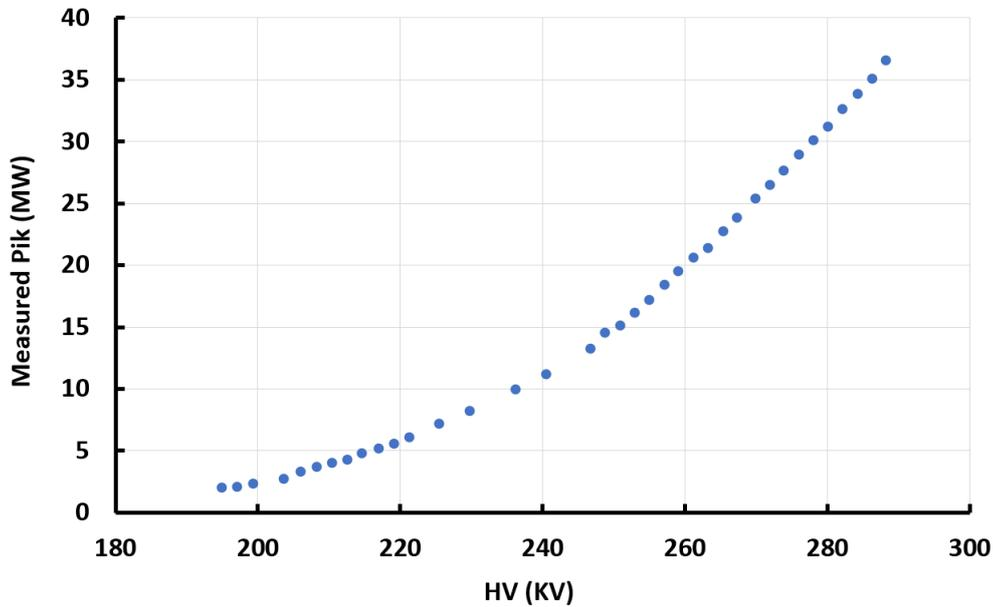
Figure 3.2:  $P_{\text{ik}}$  vs. voltage (HV) applied to Klystron.
