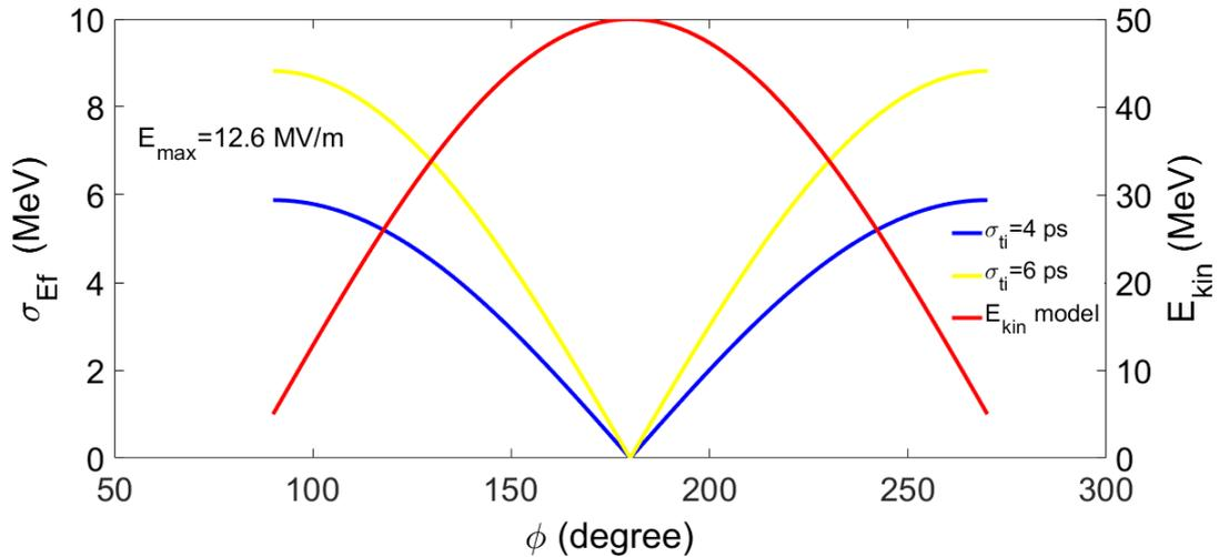
Figure 3.31: The kinetic energy  $E_{\text{kin}}$  and the energy spread  $\sigma_{\text{Ef}}$  for two bunches 4 ps and 6 ps as a function of the RF phase  $\phi$  in the LIL TW section at  $E_{\text{max}}$  12.6 MV/m.
