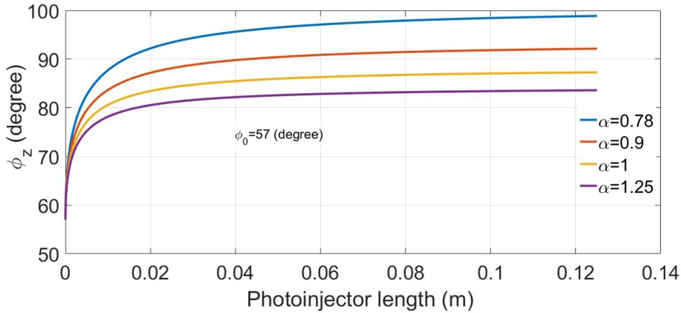
Figure 3.15: The accelerating phase  $\varphi_z$  of the electrons as a function of the photoinjector length at  $\varphi_0 = 57^\circ$  for different accelerating fields.
