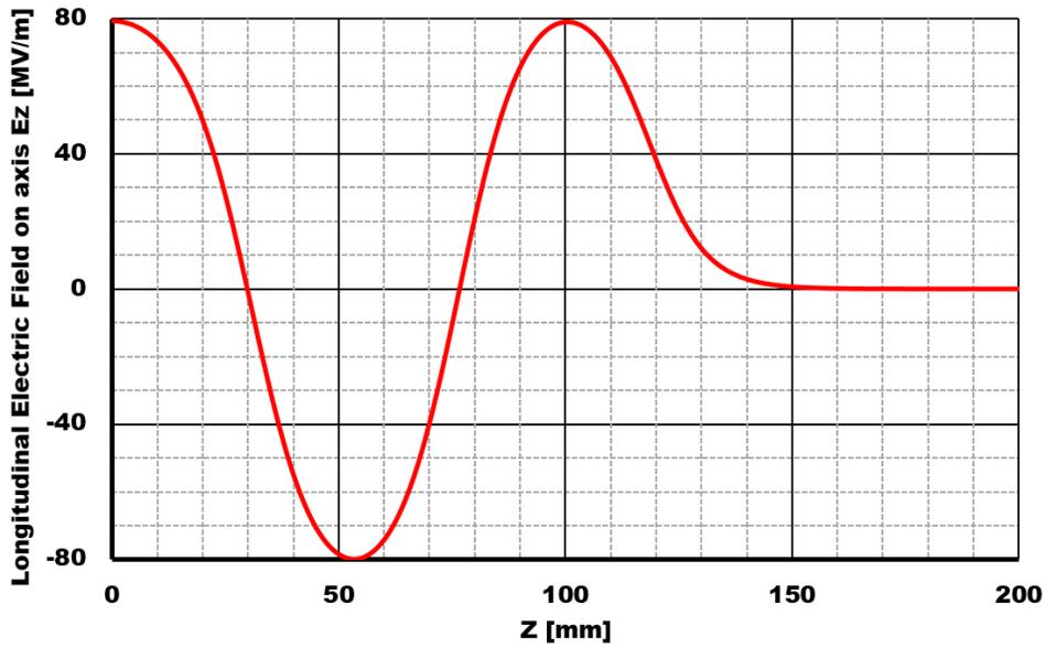
Figure 2.26: On-axis electric field for the  $\pi$ -mode ( $TM_{010-\pi}$  mode) of the ThomX RF gun with 6 MW input power.
