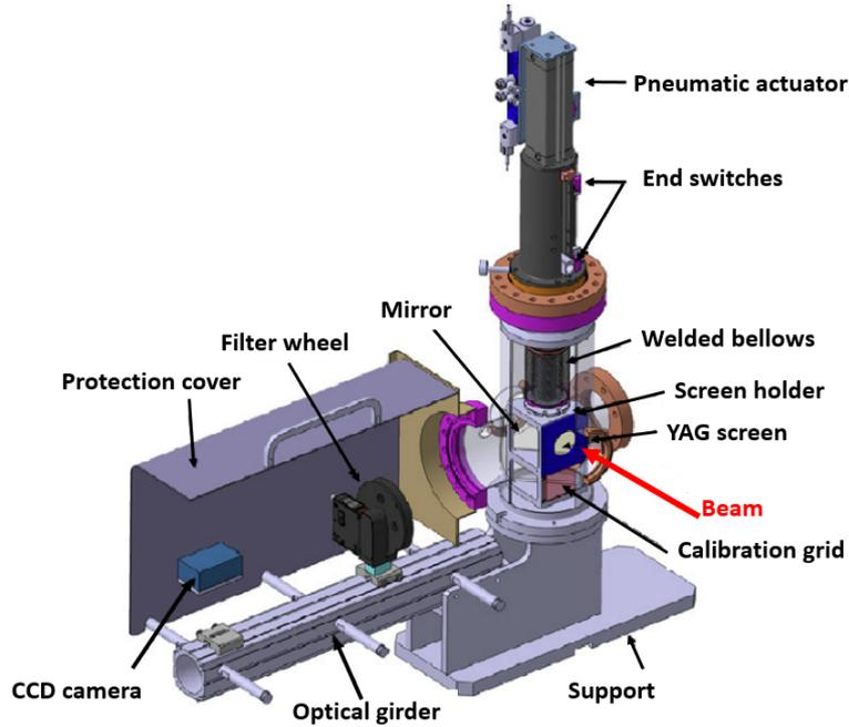
Figure 3.23: 3D view of the screen station [55].
