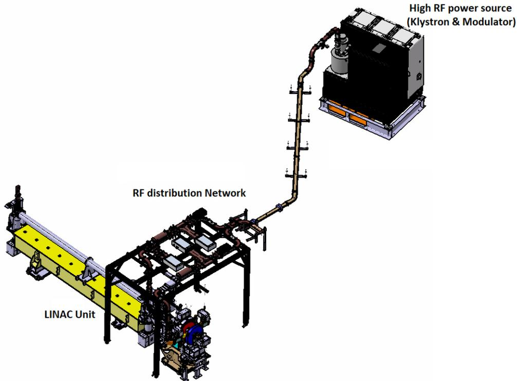
Figure 2.1: 3D model of ThomX linac.
