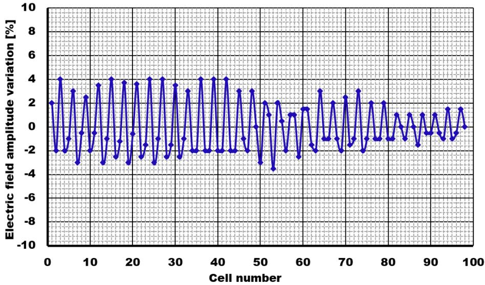
Figure 4.10: The simulated cell-to-cell axial electric field amplitude variation versus the cell number.
