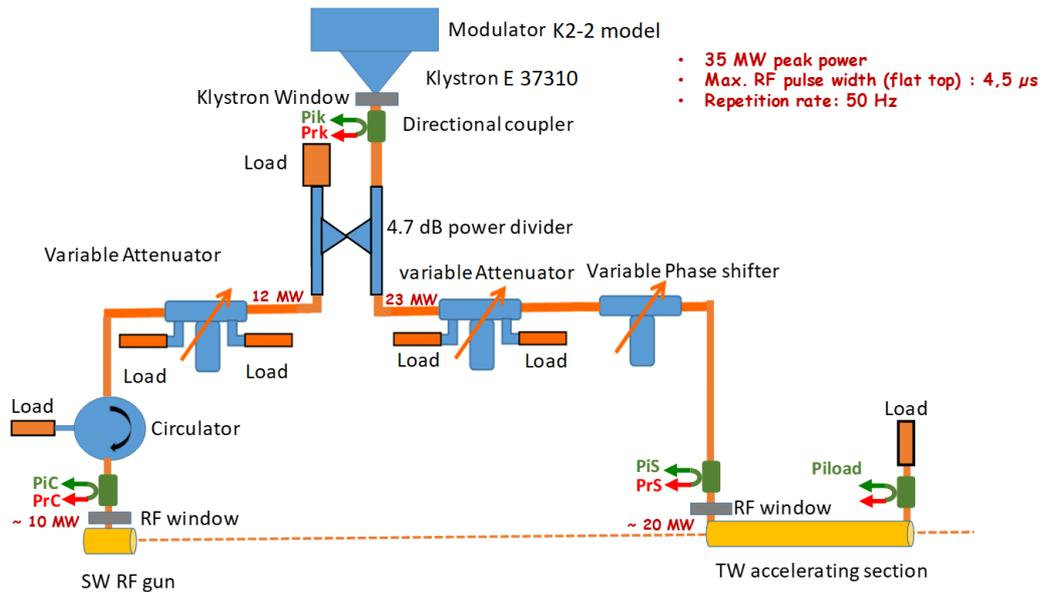
Figure 2.11: Diagram of the ThomX power distribution network.
