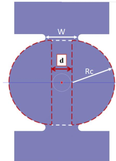
Figure 4.3: Dual-feed racetrack design of the RF coupler.
