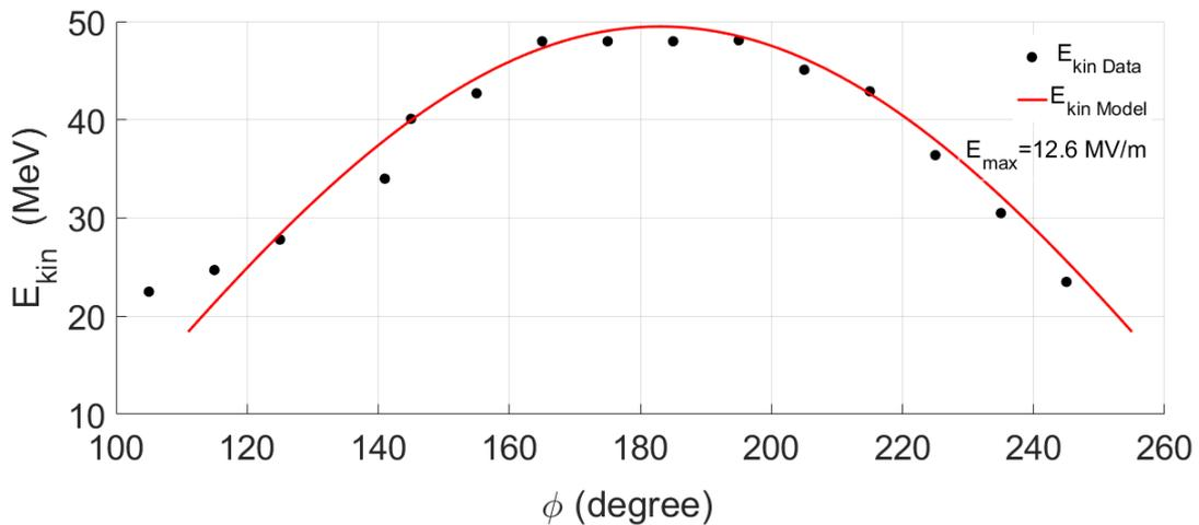
Figure 3.28: The experimental and analytical electron kinetic energy  $E_{\text{kin}}$  at the exit of the LIL structure as a function of the RF phase  $\varphi$  for  $E_{\text{max}}=12.6$  MV/m.
