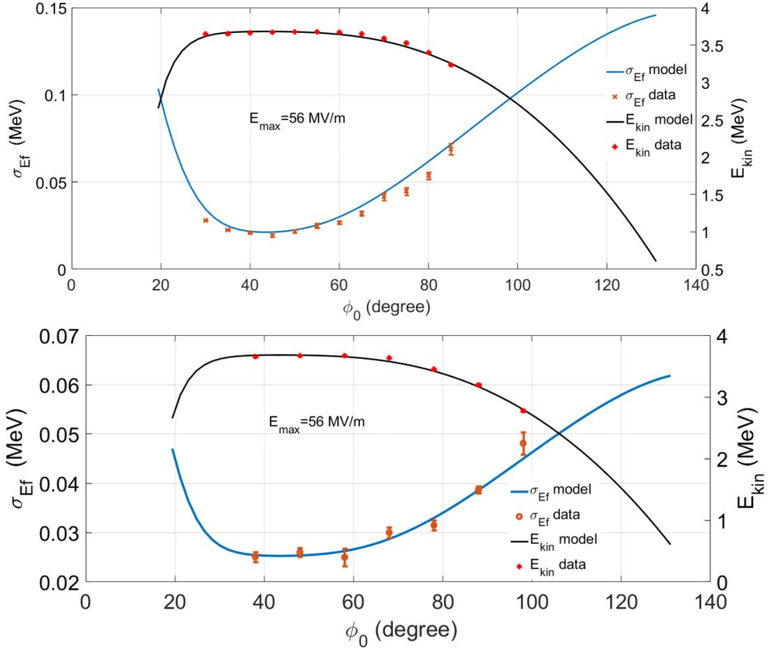
Figure 3.30: The kinetic energy  $E_{kin}$  and the energy spreads  $\sigma_{Ef}$  (model and measurement) for two electron bunches of length 3 ps (upper) and 0.6 ps (lower) as a function of RF phase  $\phi_0$  at  $E_{max}=56$  MV/m.
