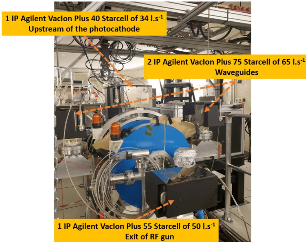
Figure 2.47: Ion pumps installed on the RF gun.
