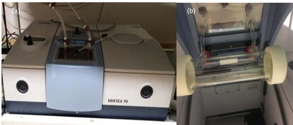
Figure 3 - 11: (a) Bruker Vertex 70 FT-IR spectrometer, (b) Gas cell
