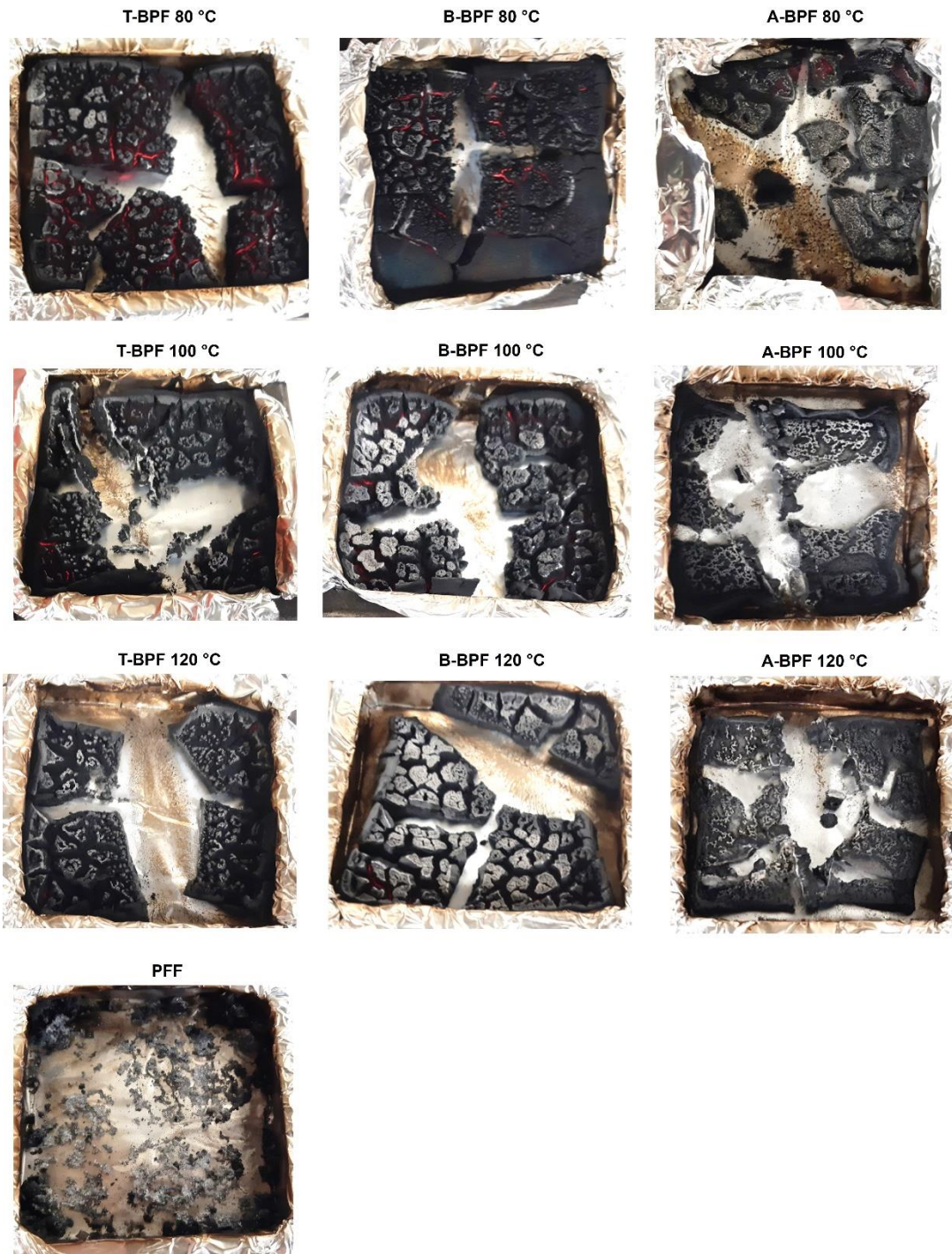
Figure S8: Photographs of residues after the cone calorimeter tests
