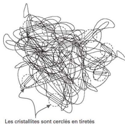
Figure I-2. Morphologie semi-cristalline (Fontanille and Gnanou, 2009).
