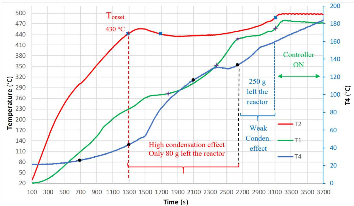
**Figure 4-26** : Temperature results of 400 g PP pyrolysis inside the semi-batch reactor of 750 W average heating power.
