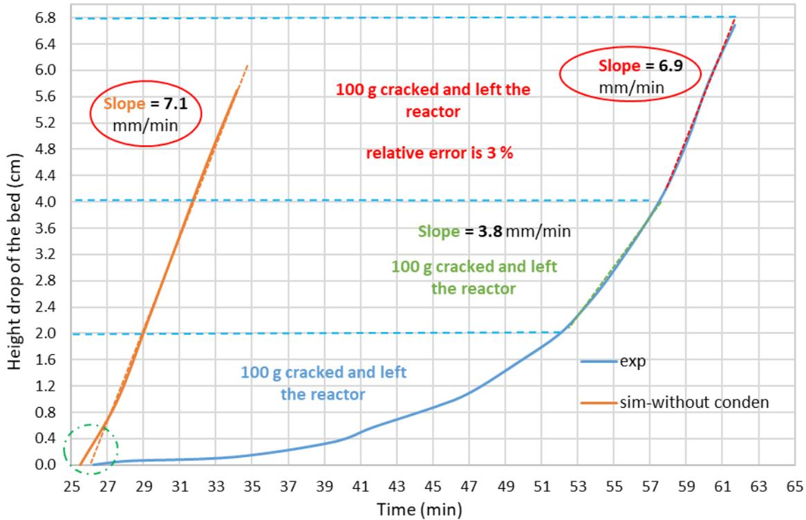
**Figure 4-30 :** Bed loss comparison between the simulated and experimental results for PP pyrolysis at 600 W heating power, without modelling the condensation process.
