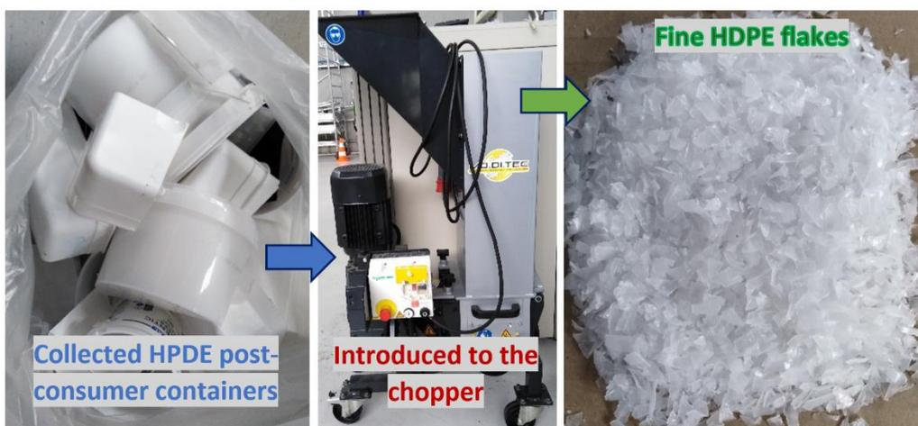
**Figure 2-2:** Preparing HDPE flakes from plastic waste containers.
