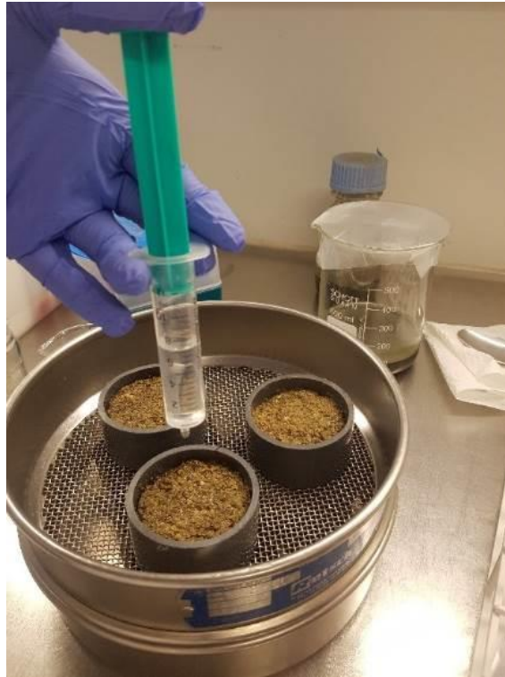
Figure V.2 Preparation of the soil runoff by mimicking rain. Soil samples subjected to rain laid on a 2 mm sieve in order to collect runoff
