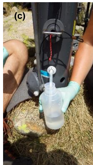
Figure 3-4: Water collection using a Go-Flo sampler ((a) subsurface; (b) deep water; (c) sub-sampling).
