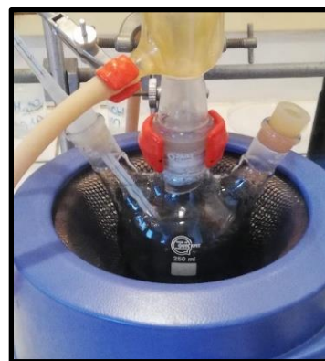
Figure 75. Heat treatment of graphene oxide with hydrazine hydrate.
