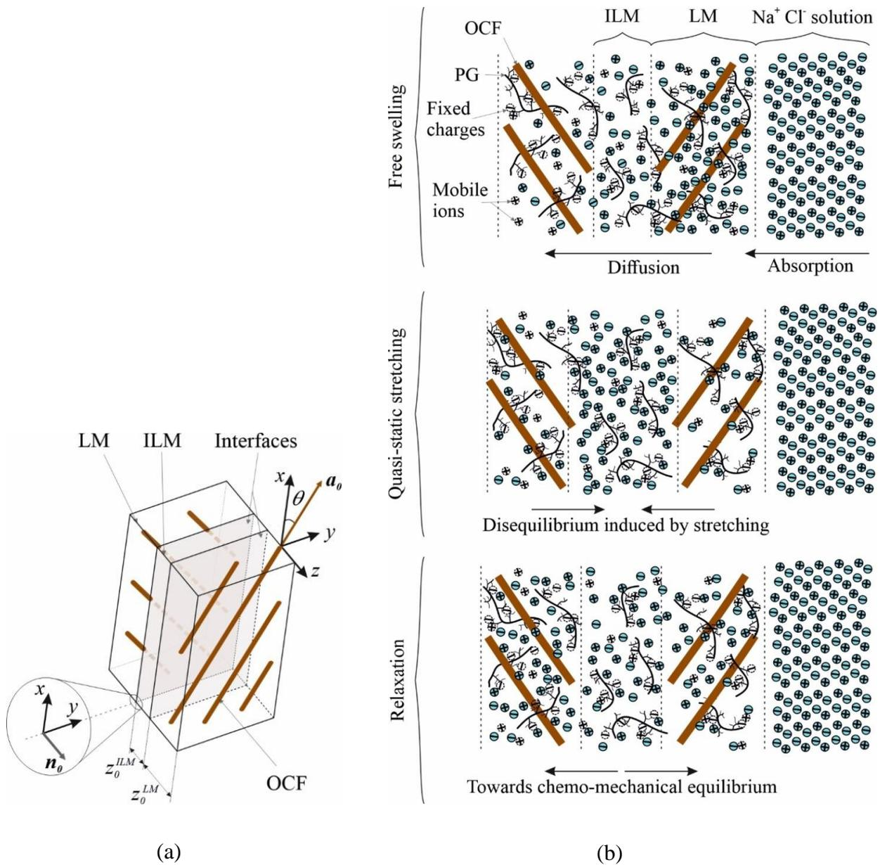
Figure I.2. Chemo-mechanical interactions: (a) Mechanical interactions between layers due to the stress/strain continuity along the interfaces (The main  $\mathbf{a}_0$ -axis of OCF in LM forms an angle  $\theta$  with
