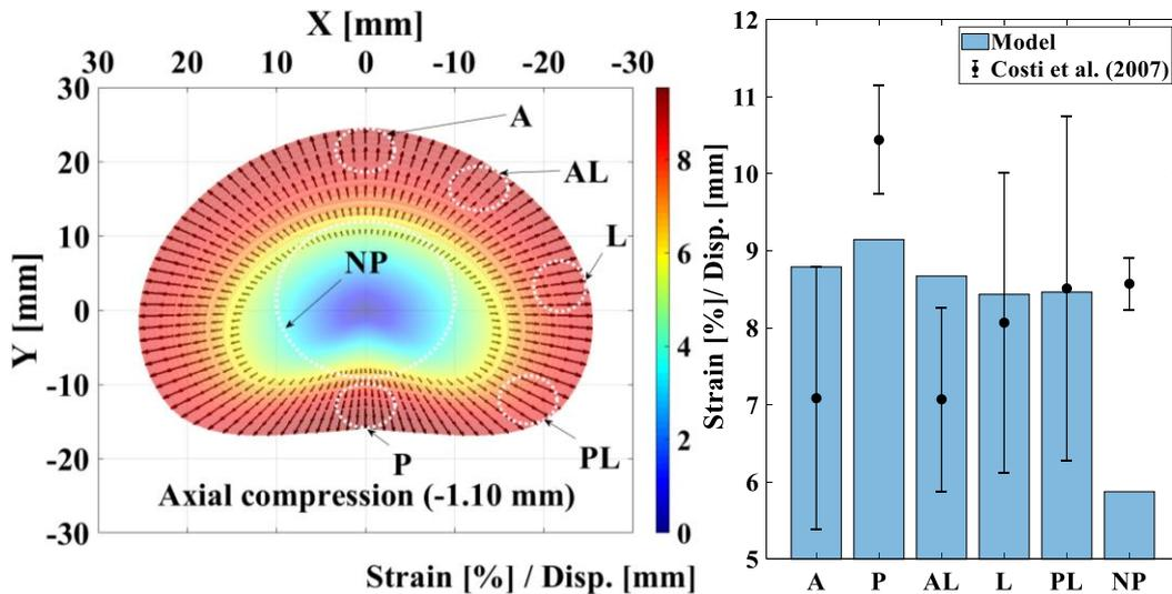
Figure IV.6. Predicted normalized radial strains (%/mm) in a disc compressed at 1.1 mm. The comparison to Costi et al. (2007) data is performed for different regions in which the local strains are averaged (A: Anterior, P: Posterior, AL: Anterior-Lateral, L: Lateral, PL: Posterior-Lateral, NP: nucleus pulposus).
