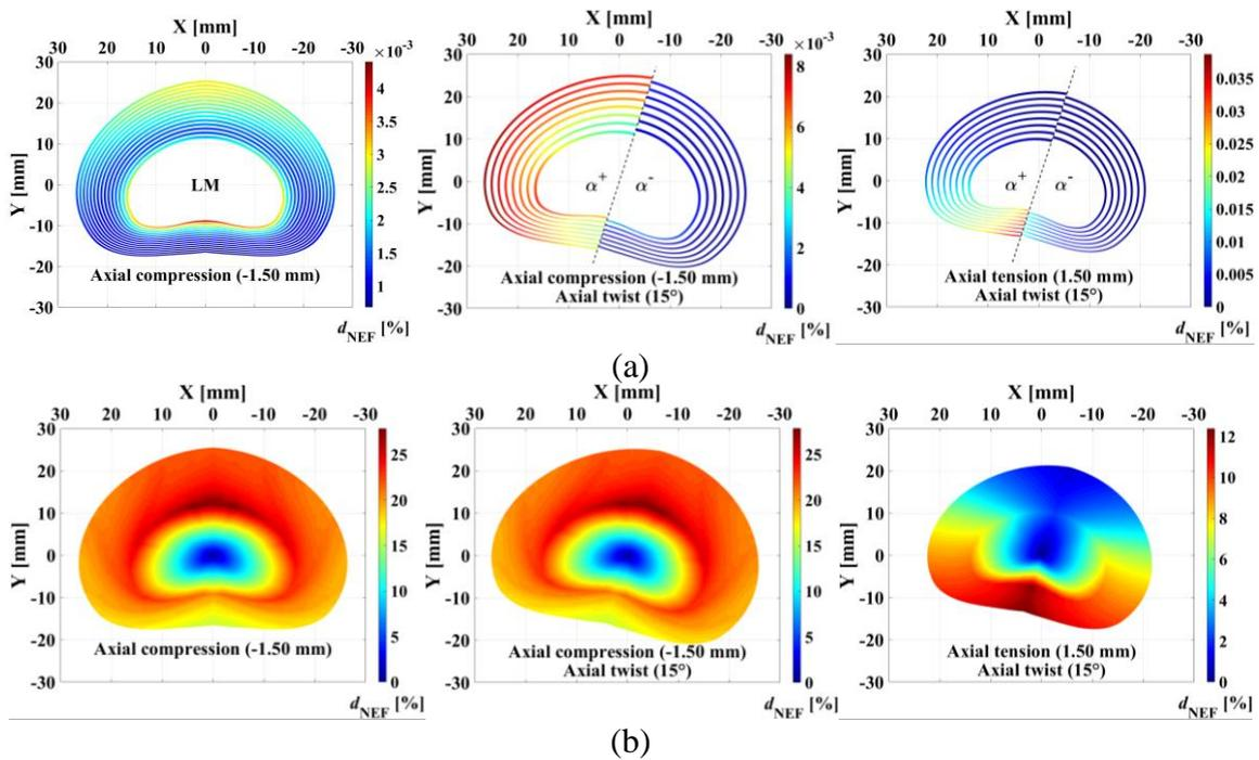
Figure IV.11. Contour plots of the NEF damage  $d_{NEF}$  in axially/torsionally loaded discs: (a) in LM, (b) in ILM.
