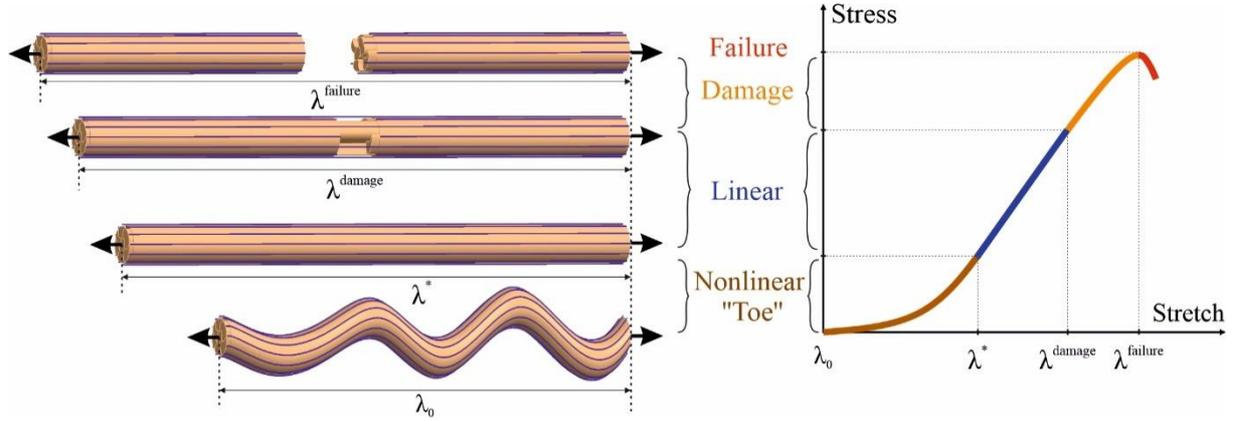
Figure II.4. Behavior of a single collagen fiber stretched until failure.
