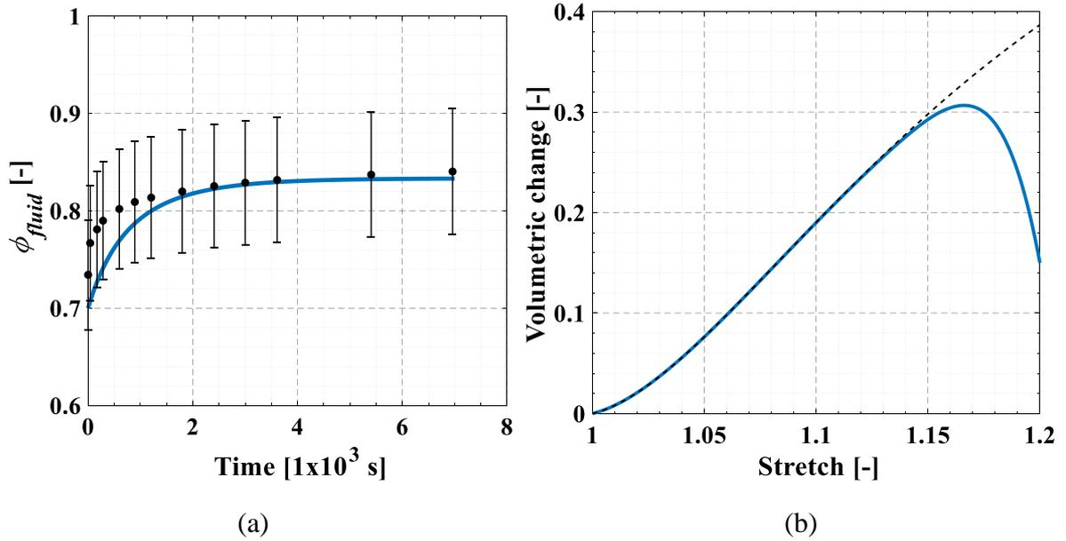
Figure II.6. Volumetric response of the multi-layered material element: (a) under free swelling (line: model, symbol: experimental data of Acaroglu et al. (1995)), (b) under UA circumferential stretching (solid line: model, dashed line model without damage).
