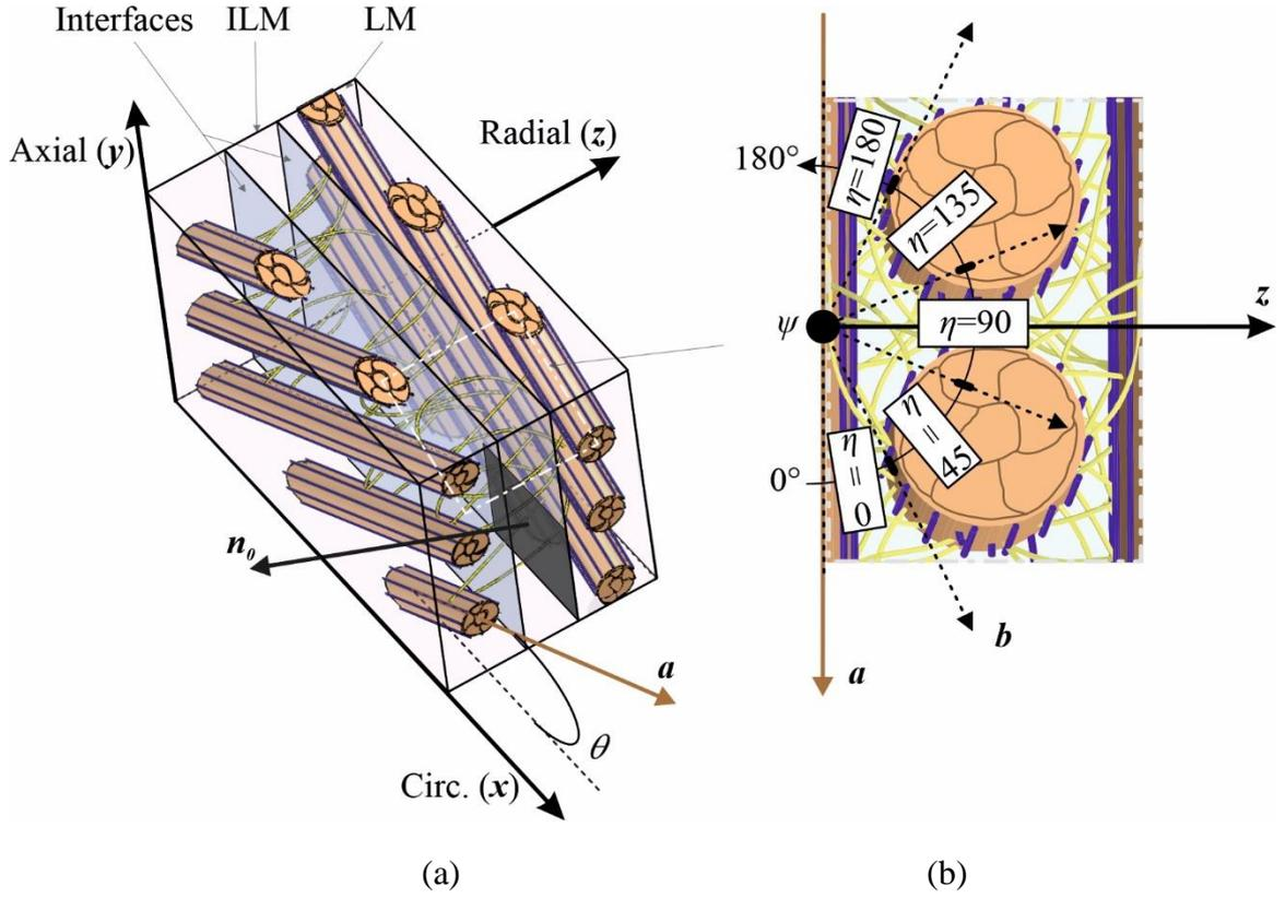
Figure II.2. Coordinate systems of (a) the multi-layered material element ( $n_0$ -axis is the unit vector at inter-layer interfaces and  $a$ -axis is the unit vector along OCF that forms an angle  $\theta$  with the  $x$ -axis) and (b) of the five NEF bundles  $\eta = \{0^\circ, 45^\circ, 90^\circ, 135^\circ, 180^\circ\}$  ( $b$ -axis is the unit vector along NEF that forms an angle  $\psi$  with the  $a$ -axis).
