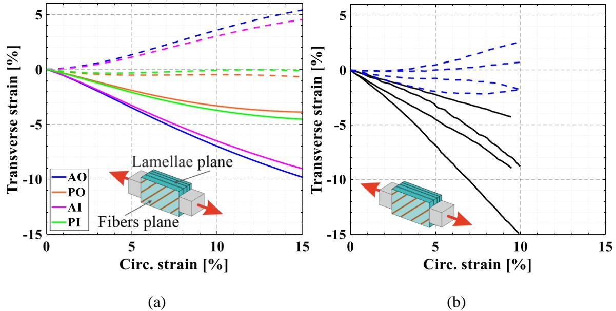
Figure III.6. Multi-lamellae transverse responses under UA circumferential stretching for the different disc regions (solid lines: fibers plane, dashed lines: lamellae plane): (a) model results, (b) experimental data of Baldit (2013).
