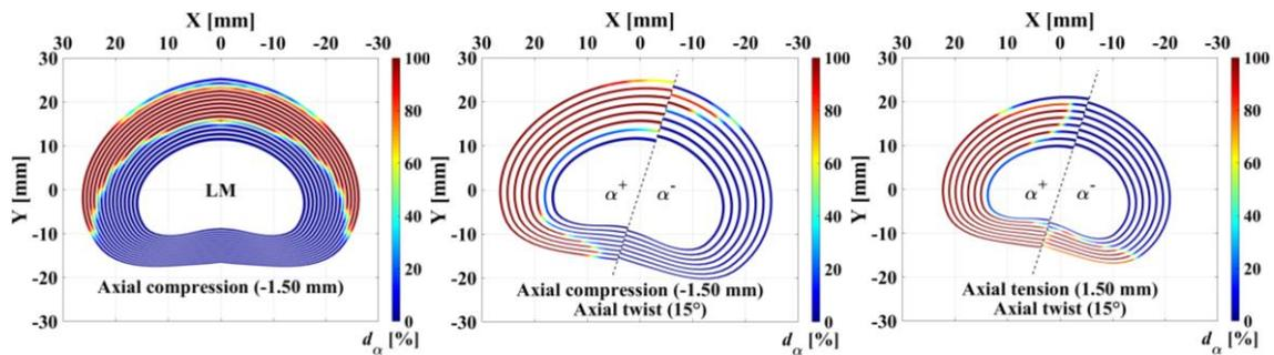
Figure IV.12. Contour plots of the OCF damage  $d_{\alpha}$  (in LM) in axially/torsionally loaded discs.
