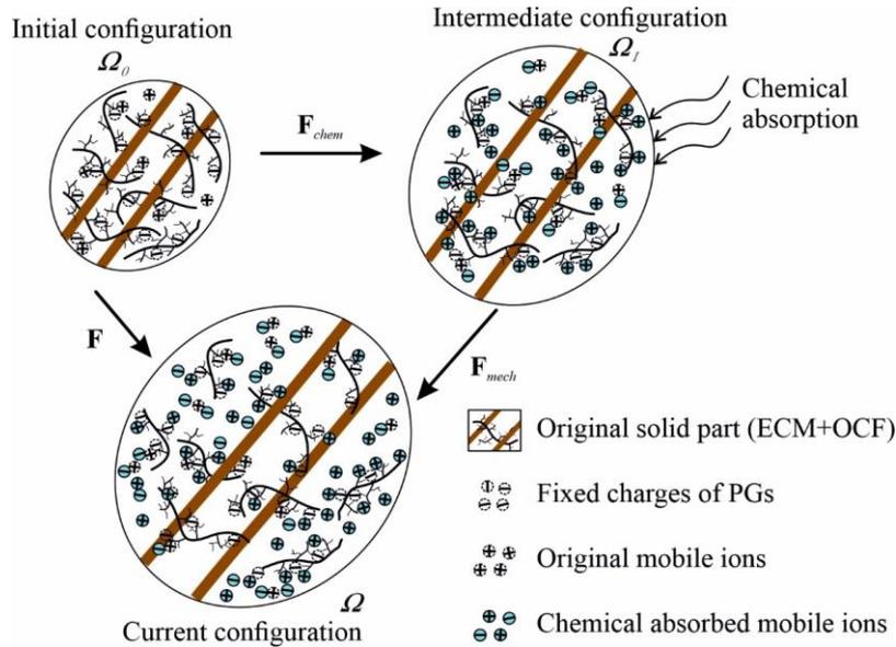
Figure I.1. Decomposition of the deformation gradient  $\mathbf{F}$  into chemically-induced fluid transfer part  $\mathbf{F}_{chem}$  and purely mechanical part  $\mathbf{F}_{mech}$ .
