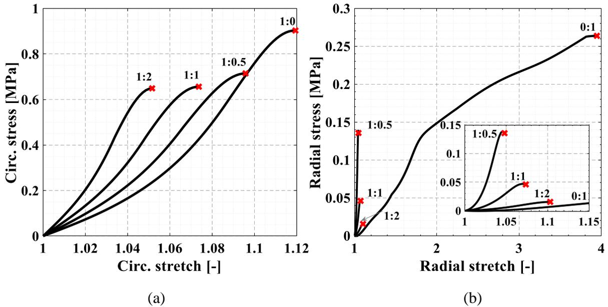
Figure II.12. Biaxial stretching of the multi-layered material element for different biaxiality ratios: (a) circumferential stress-stretch response, (b) radial stress-stretch response.
