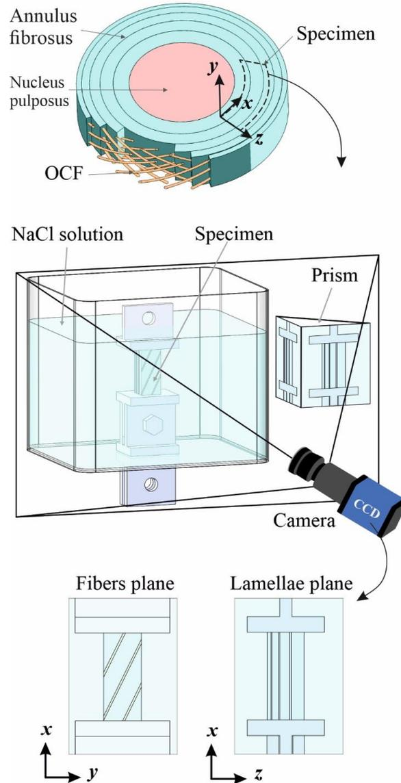
Figure I.3 Annulus specimen extracted from intervertebral disc and stretched in the circumferential direction  $x$  with simultaneous local displacement measurements in fibers plane  $xy$  and in lamellae plane  $xz$  using a right-angle prism.
