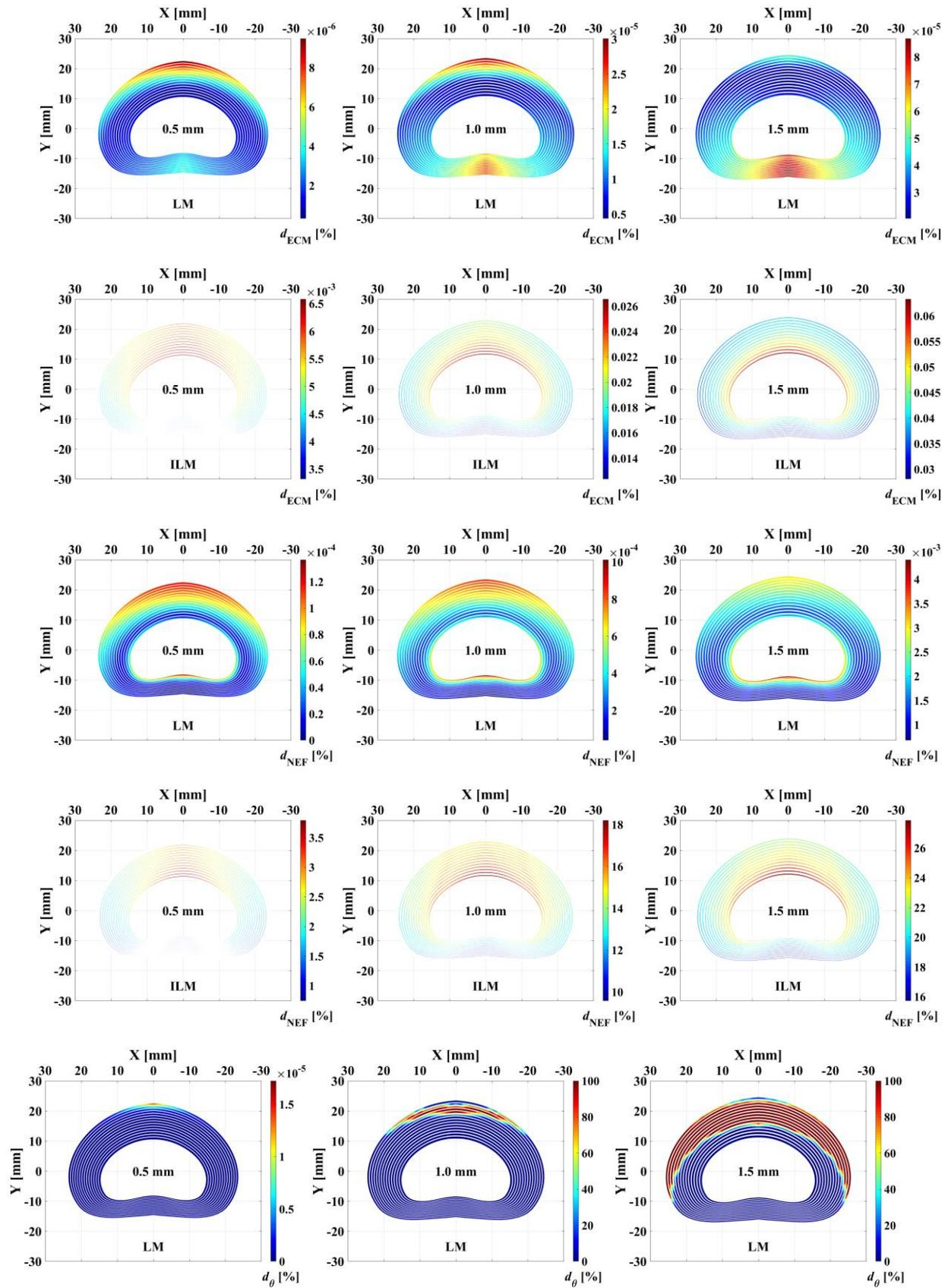
Figure III.12. Damage contour plots in the superior view of the uniaxially compressed disc for different applied displacement levels (0.5, 1.0 and 1.5 mm); ECM damage  $d_{ECM}$  in LM and in ILM, NEF damage  $d_{NEF}$  in LM and in ILM, OCF damage  $d_{\theta}$  in LM.
