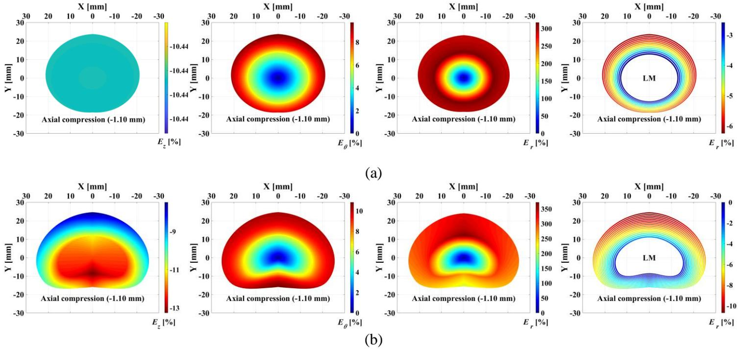
Figure IV.9. Morphology influence on the local strains local axial, circumferential and radial strains  $E_z$ ,  $E_\theta$  and  $E_r$  (in ILM and in LM) in axially compressed discs: (a) simplified disc morphology in circular basis with  $R_{sagittal}^0 = R_{frontal}^0$  (all initial heights and OCF orientations in Table IV.1 are averaged), (b) actual disc morphology.
