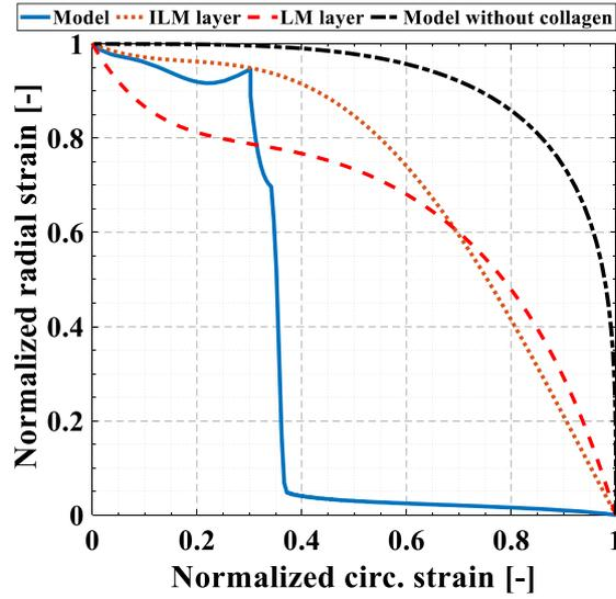
Figure II.13. Biaxial failure envelope.
