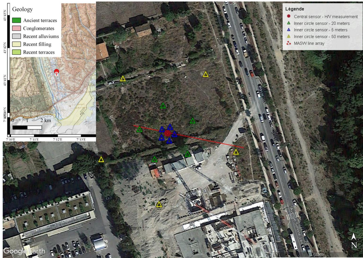
Figure 79: Localization of the MASW and AVA arrays in the LVV.
