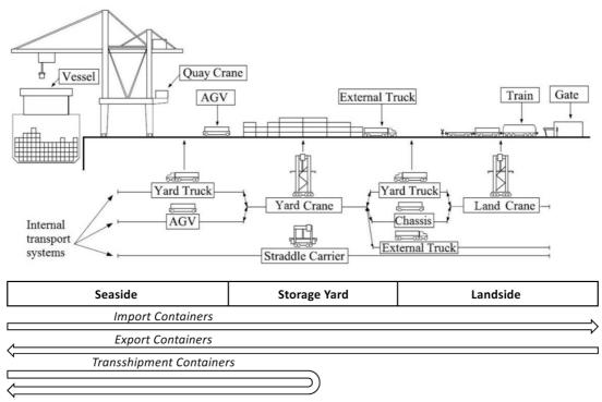
Figure 1.4: Schematic representation of a container terminal (Galle, 2018)
