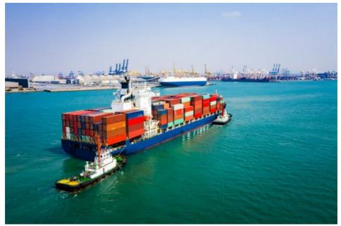
Figure 2.5: Tugboats assisting a container ship<sup>5</sup>
