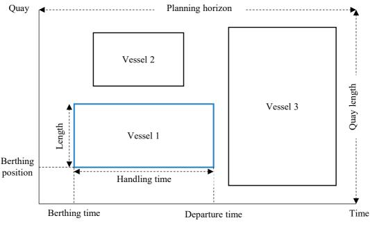
Figure 2.1: Graphic representation of a berth plan
