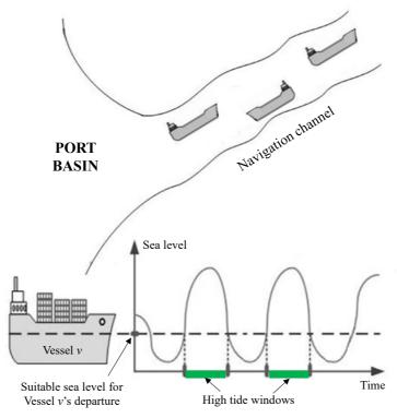
Figure 2.3: Navigation channel restrictions
