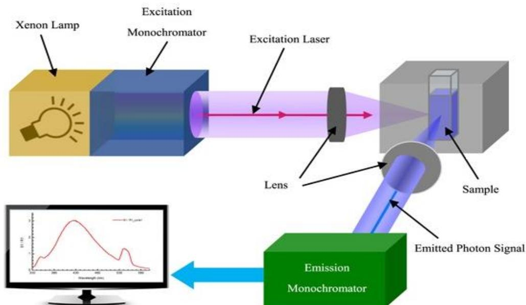
**Figure 5:** Schematic representation of fluorescent spectroscopy [4].
