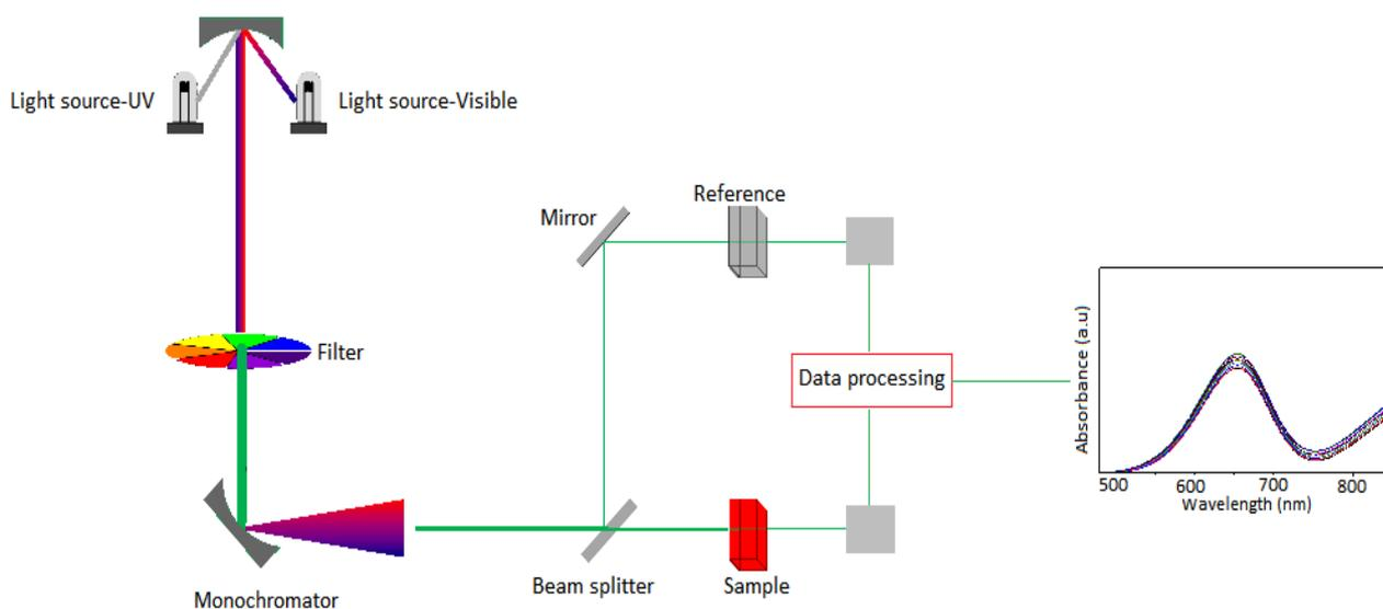
**Figure 4:** Schematic diagram of a UV-Vis spectrophotometer.
