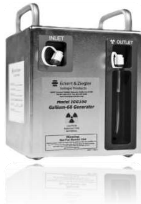
Figure 8 ^{68}\text{Ge}/^{68}\text{Ga} generator Eckert & Ziegler IGG 100
