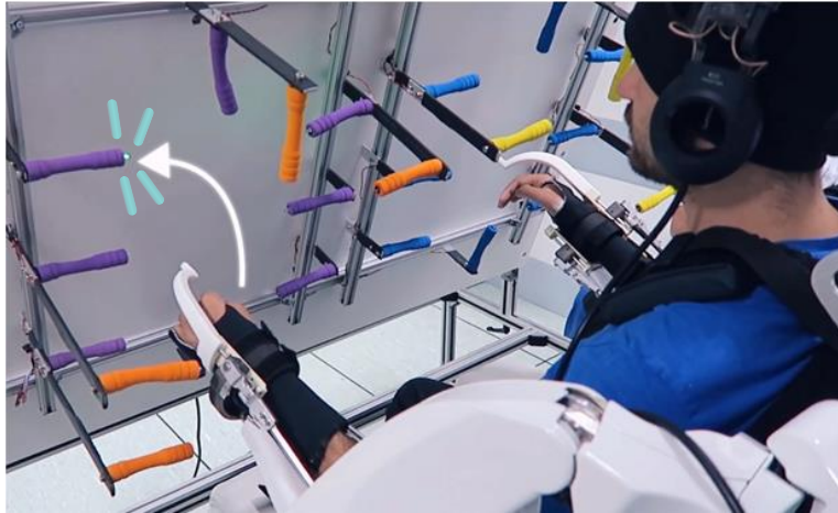
Figure 7 Environment used for the training of the decoders used to move the hands of the exoskeleton in 3D. At any time, one LED was turned on and the subject had to try to reach the LED using motor imagery.
