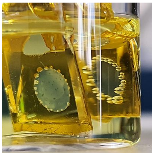
Figure 39: Simultaneous deposition and operation of the dual catalysts by a 3jn-a-Si under illumination
