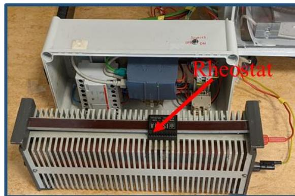
Fig 5.16. Rheostat used for emulating faults in panel.
