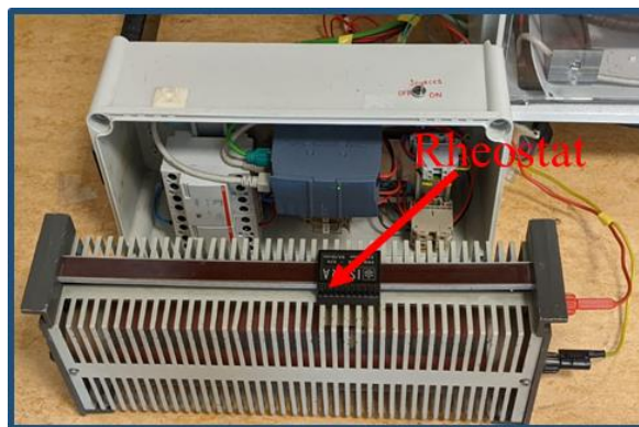
Fig 5.16. Rheostat used for emulating faults in panel.
