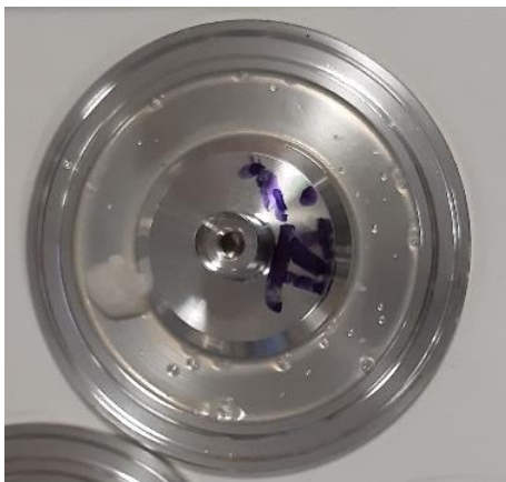
Figure 2.21. Test with spilled reactive mix.
