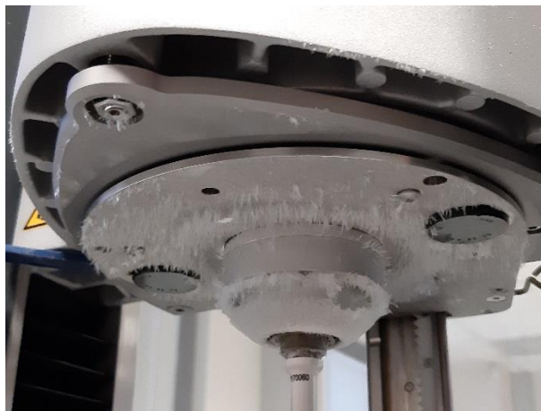
Figure 2.22. Reactants formed by condensation observed above the rheological test (Haake Mars 60 rheometer).
