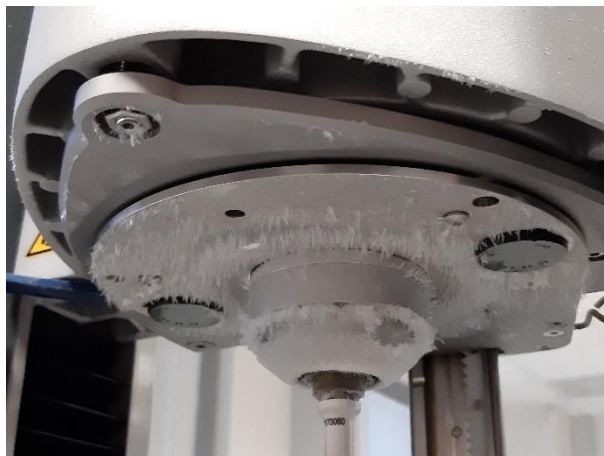
Figure 2.22. Reactants formed by condensation observed above the rheological test (Haake Mars 60 rheometer).
