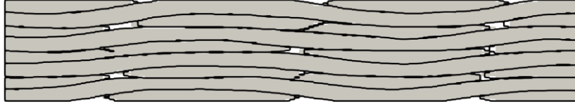
Figure 1.33. Comparison between 3D geometry tow geometry (black borders) and tows zone in the meshing (grey). Position of the cross-section is described in Figure 1.23.
