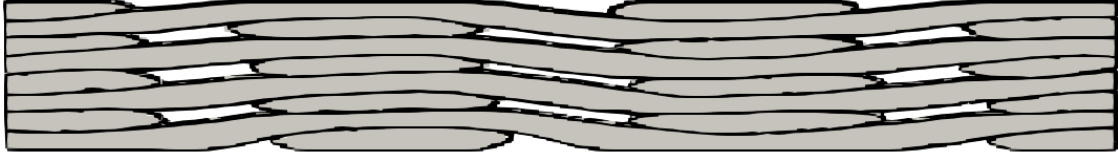
Figure 1.32. Comparison between 3D geometry tow geometry (black borders) and tows zone in the meshing (grey). Position of the cross-section is described in Figure 1.22.
