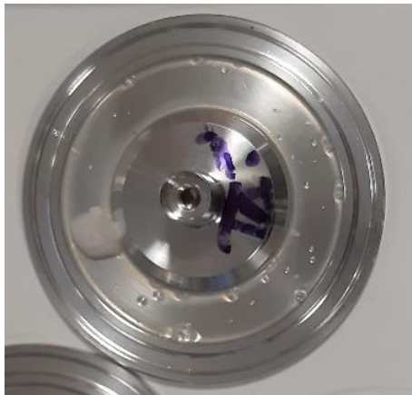
Figure 2.21. Test with spilled reactive mix.
