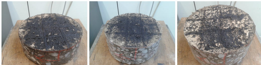
(a) Dirt on BC of specimen 452-7: degree 1 (b) Dirt on BC of specimen 453-3: degree 2 (c) Dirt on BC of specimen 4W3-1: degree 3
