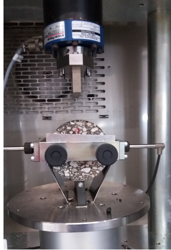
Figure III.4.2: Test specimen inserted in the fatigue testing device
