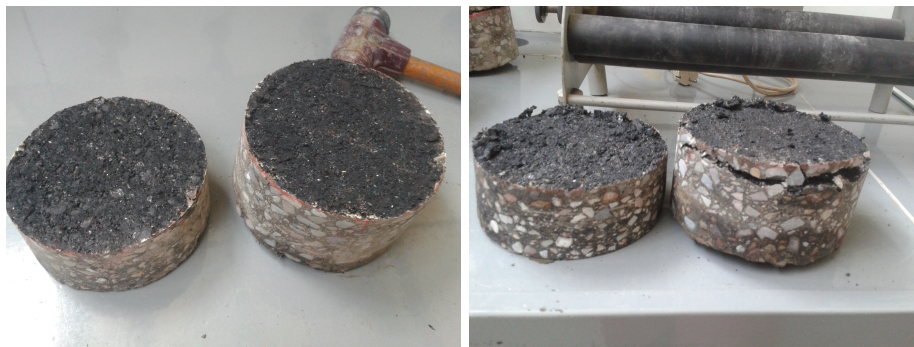
(a) Interface as it should be (Specimen 601-1) (b) Pullout on the side of a specimen (602-4)
