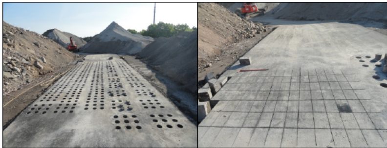
Figure III.1.4: Test surface after the extraction of the specimens
