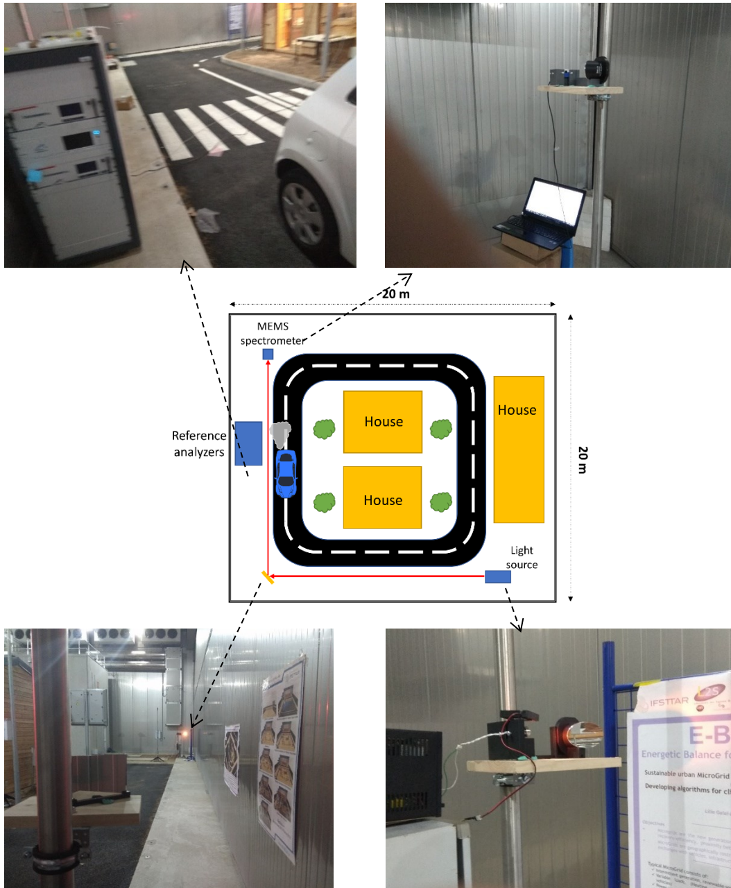
Figure 3-5 Top schematic view of Sense city for air pollution monitoring using open-path FTIR in addition to camera photos in different positions inside the city.
