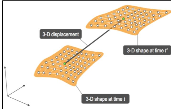
**Figure 22 : Deformation tracking via digital image correlation**
