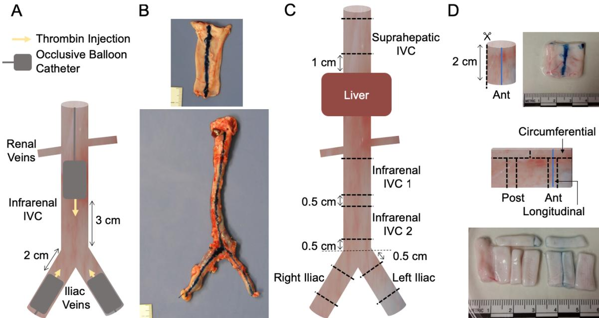
**Figure 14 : Samples preparation for mechanical testing**
