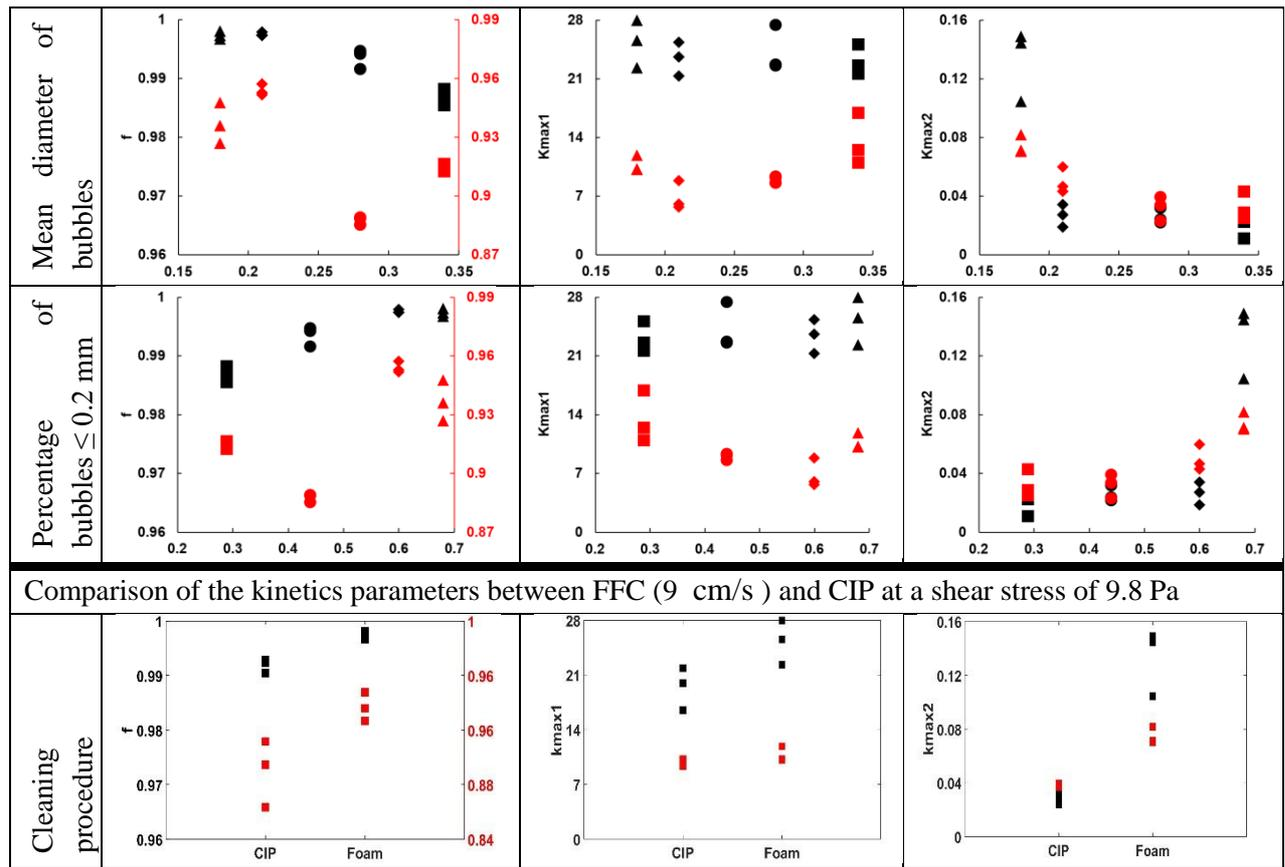
**Figure 69.** Variations induced on the kinetics parameters  $f$ ,  $K_{max1}$  and  $K_{max2}$  for *B. subtilis* PY79 (black color) and *B. subtilis* PY79 *spcA* (red color) spores under different flow conditions: 1.5 cm/s (square), 4.5 cm/s (circle), 9 cm/s (triangle), 13.5 cm/s (diamond), and CIP.
