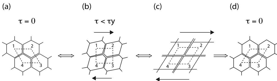
**Figure 11.** Topological rearrangement T1: Foam yielding and plastic deformation, under applied shear stress, increasing from (a) to (c). This structure can relax either elastically, by returning to structure (a), or by a bubble rearrangement, leading to structure (d) (inspired from (Princen, 1985)).
