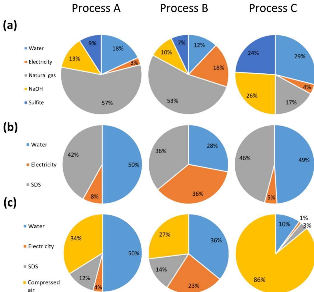
**Figure 85.** Contributors for three impact categories of the cleaning processes according to the impact assessment methods IMPACT 2002+. (a) global warming, (b) non-renewable energy, and (c) aquatic eutrophication.
