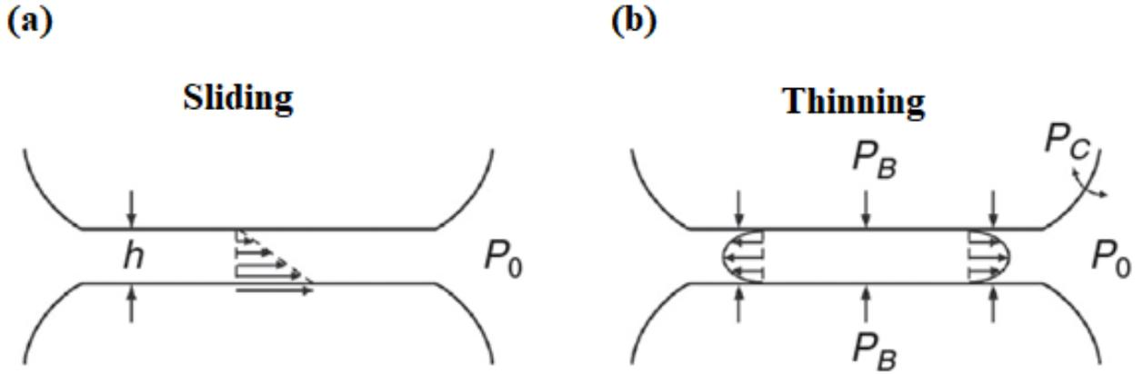
**Figure 15.** (a): Schematic presentation of the sliding process: the opposing surfaces of the film move at velocities which are driven by the relative motion of the neighboring bubbles in the flowing foam. The film thickness  $h$  determines the local shear rate of the liquid in the film. (b): Schematic presentation of the thinning of the film. This process is driven by the excess pressure  $P_B$  in the bubbles compared to the pressure  $P_0$  in the liquid outside the film.
