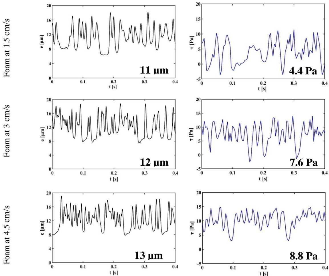
**Figure 64.** Example of the evolution of wall film thickness (left) and wall shear stress (right) given by the temporal signals of conductivity and polarography over the top wall for the three cases, respectively. The values indicated in the images show the mean thickness and the mean wall shear stress during 40 seconds of acquisition.
