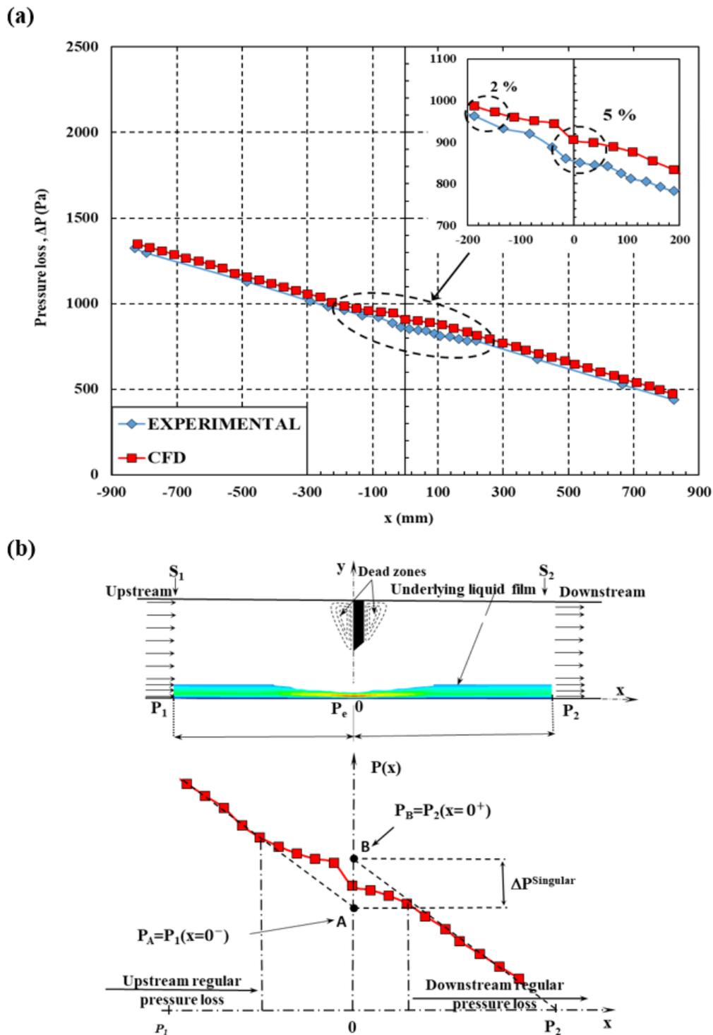
**Figure 43.** Longitudinal static pressure drop of the foam flow at  $Re = 32$ . (a): Evolution of the longitudinal static pressure drop along the test channel. (b): Zoom on the area influenced by the fence.
