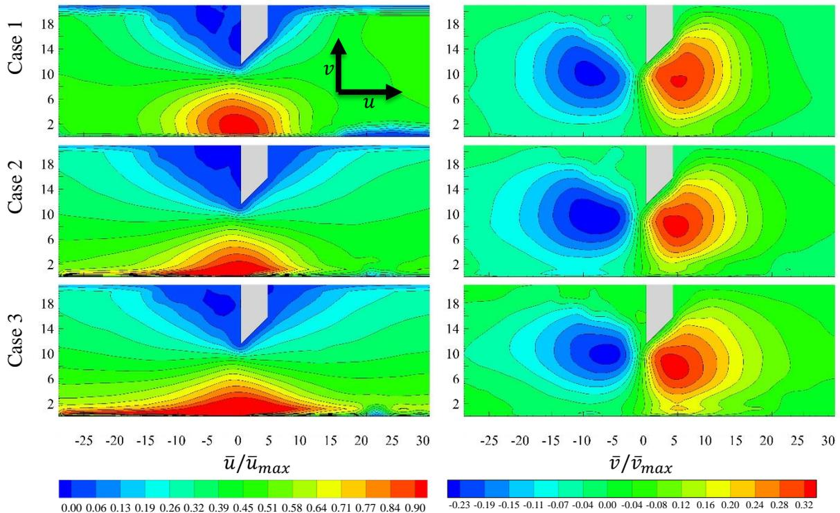
**Figure 38.** Averaged axial ( $u$ ), and vertical ( $v$ ) mean velocity components' fields for all cases under the fence. Velocity measurements were obtained using the PIV technique.  $u_{max}$  was 4.3, 9, and 14  $\text{cm}\cdot\text{s}^{-1}$  and  $v_{max}$  was 1.3, 2.2, and 2.4  $\text{cm}\cdot\text{s}^{-1}$  for cases 1,2 respectively.
