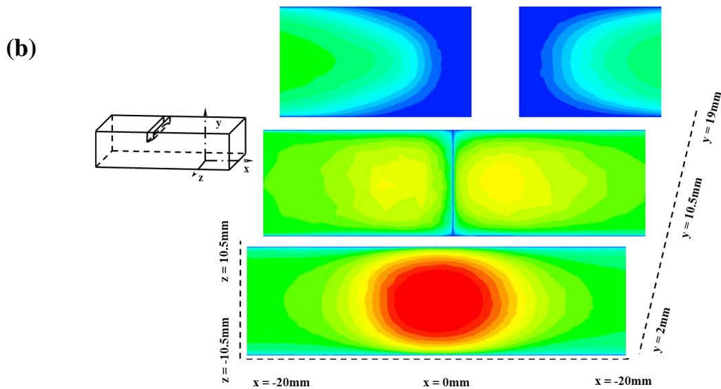
**Figure 50.** CFD spanwise (top side) axial velocity at different locations in the vicinity of the singularity for case of foam at  $Re = 97$ . (a): averaged axial velocity component profiles. (b): Axial velocity component distribution for three horizontal planes locate at:  $y = 2, 10.5,$  and  $19$  mm.
