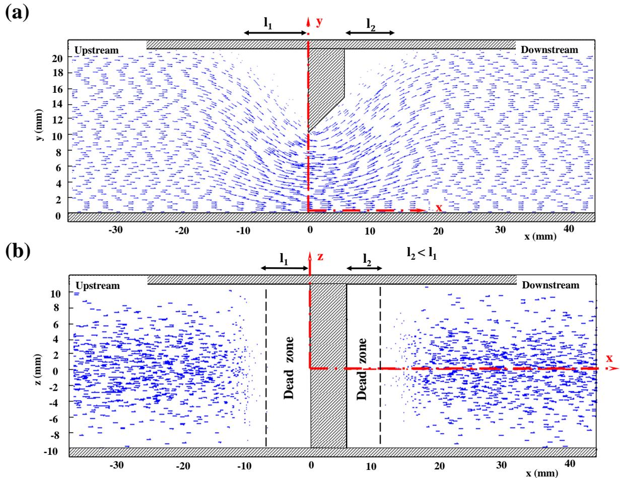
**Figure 44.** Example of velocity field obtained under the fence at the middle axis of the duct by CFD simulation using the Herschel-Bulkley model (foam at  $Re = 32$ ). (a): Lateral view. (b): Top view at  $y = 19$  mm.
