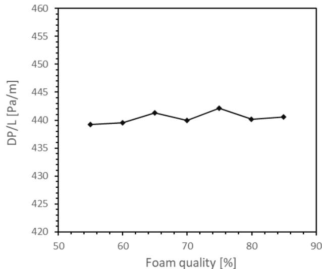
**Figure 22.** Static pressure gradient for a foam flow inside a straight channel for different foam qualities.
