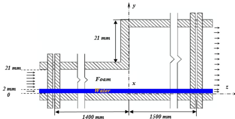
**Figure 28.** Lateral view of the of the half-sudden expansion.
