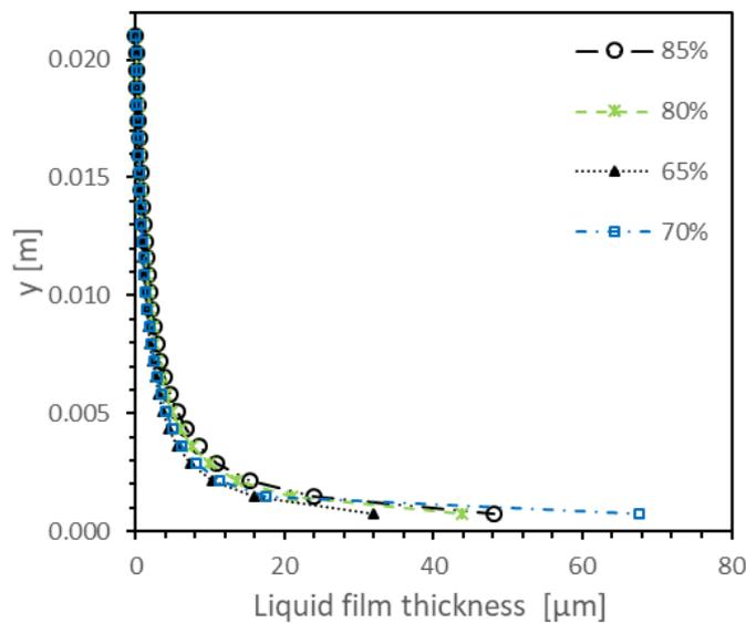
**Figure 25.** Estimation of the liquid film thickness the evolution on the lateral wall for all studied foam qualities  $\beta$ .
