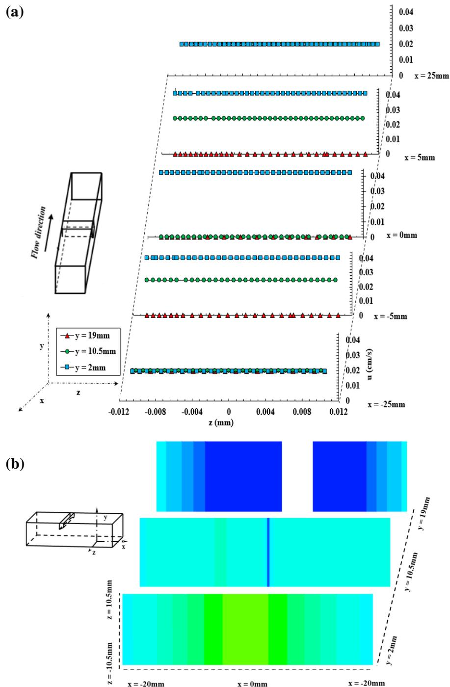
**Supplementary data 4- Figure 47.** CFD spanwise (top side) axial velocity at different locations in the vicinity of the singularity for case 1. (a): averaged axial velocity component profiles. (b): Axial velocity component distribution for three horizontal planes located at:  $y = 2$ ,  $10.5$ , and  $19$  mm.
