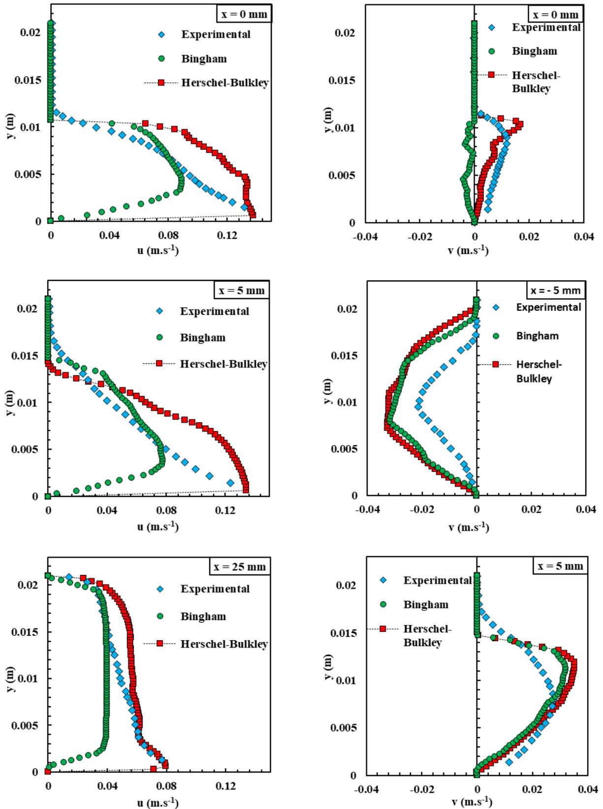
**Figure 49.** Lateral averaged axial ( $u$ ) and vertical ( $v$ ) mean component velocity profiles for different positions near the singularity, for the case of foam at  $Re = 97$  and different rheological models.
