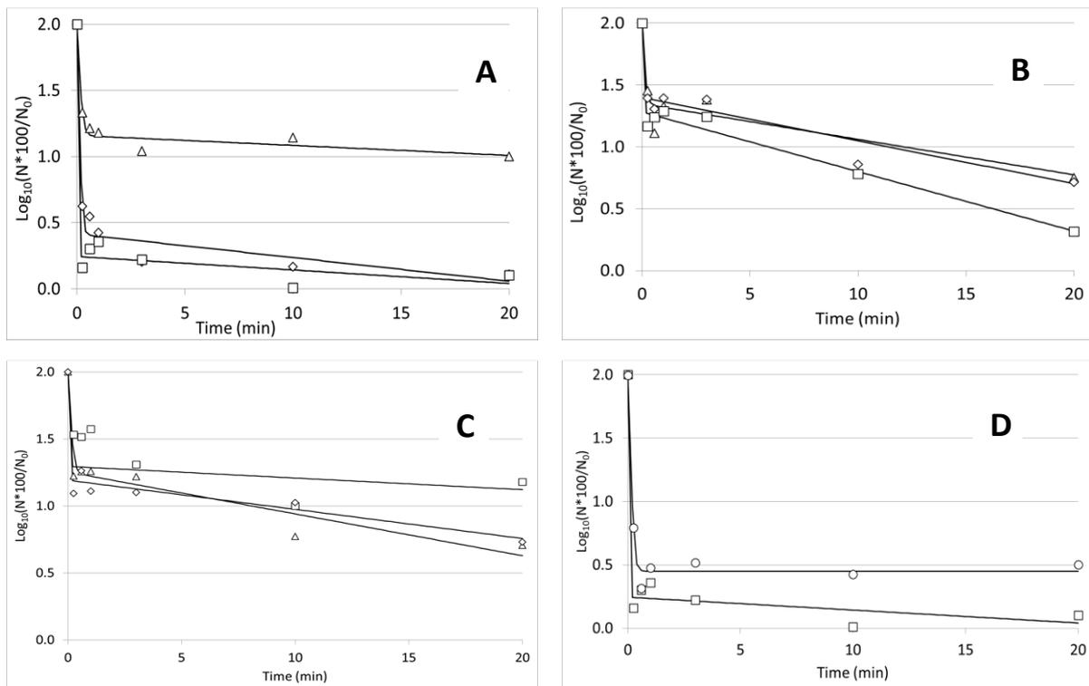
**Figure 55.** Removal kinetics of *B. amyloliquefaciens* 98/7 spores under different flowing conditions: 1 generator (square), 2 generators (diamond), 3 generators (triangle) for the foam qualities of 50% (A), 60% (B) and 70% (C); Removal kinetics with the foam 50%, one generator compared to CIP (D).
