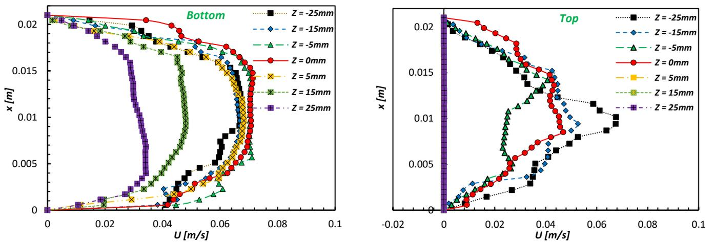
**Figure 35.** Span wise (top side) axial mean velocity profiles for different qualities and distances over the singularity.
