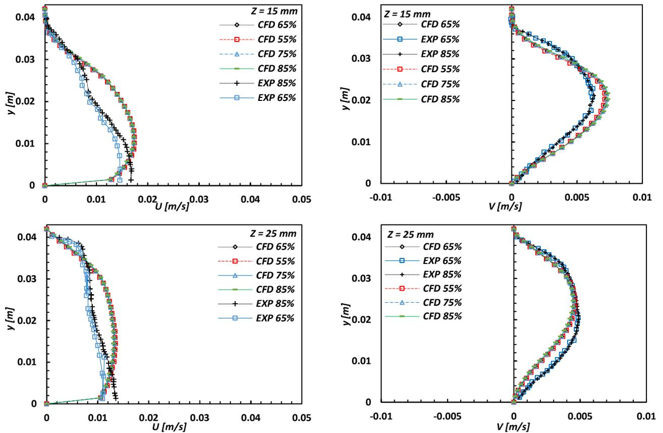
**Figure 32.** Lateral averaged axial and vertical mean velocity profiles for different qualities and distances over the singularity.
