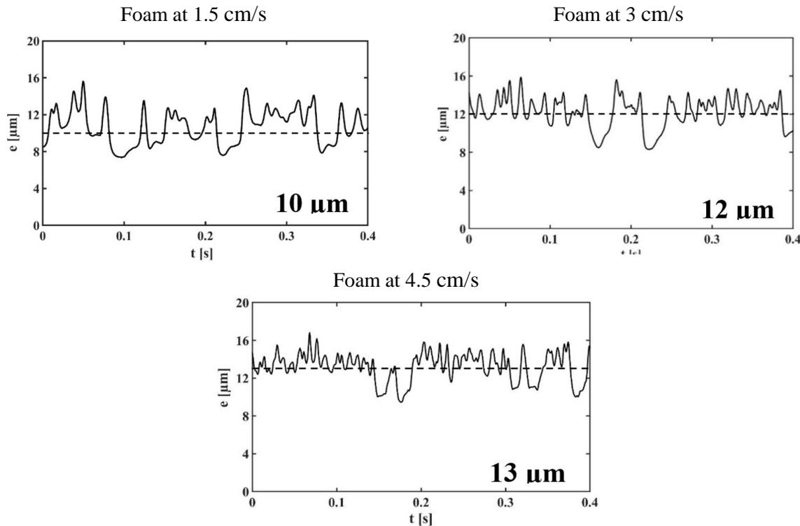
**Supplementary- Figure 65.** Example of the evolution of wall film thickness given by the temporal signals of conductimetry over the top wall for the three cases, using Ammonyx surfactant. The values indicated in the images show the mean thickness during 40 seconds of acquisition.
