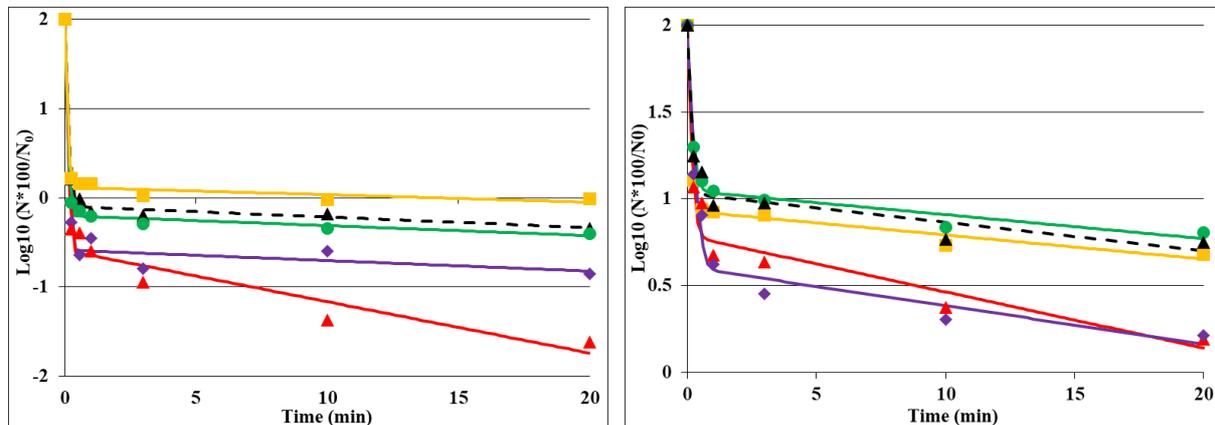
**Figure 67.** Removal kinetics of *B. subtilis* PY79 (left) and *B. subtilis* PY79 *spsA* spores under the different flow conditions. Markers showed the data of three repetitions, and the line represents the biphasic fitted model fit to each condition: 1.5 cm/s (yellow square), 4.5 cm/s (green circle), 9 cm/s (red triangle), 13.5 cm/s (purple diamond), and CIP (black triangle).
