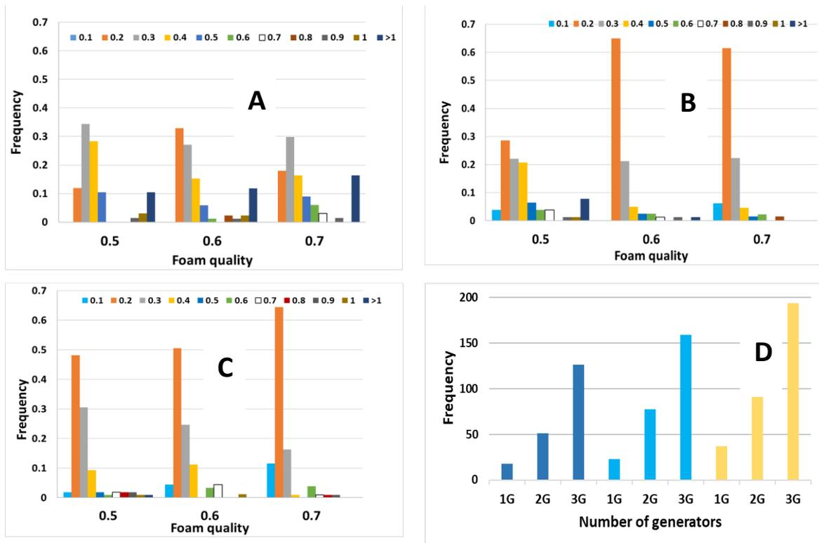
**Figure 54.** Bubble size (mm) repartition; A: one generator, B: 2 generators & C: 3 generators and frequency of passage of bubbles in front of the optical probe (D) at the top wall for the three foam qualities: 0.5 (dark blue), 0.6 (light blue), 0.7 (yellow).
