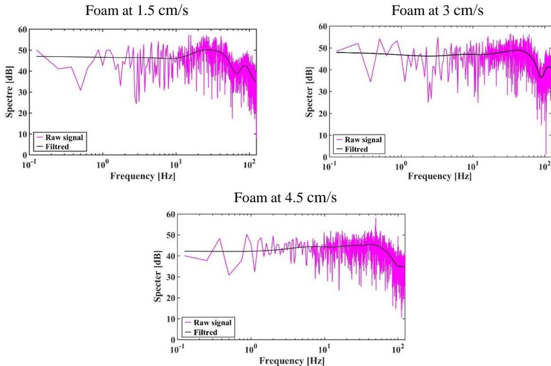
**Supplementary- Figure 66.** Example of spectral densities of the velocity gradient measured using polarography method for the three cases. This spectrum presentation provides for the identification of the characteristic frequencies corresponding to the passage frequencies of bubbles using Py. (1990) method.
