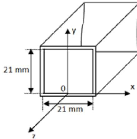
**Figure 20.** 3D geometry of test-section.
