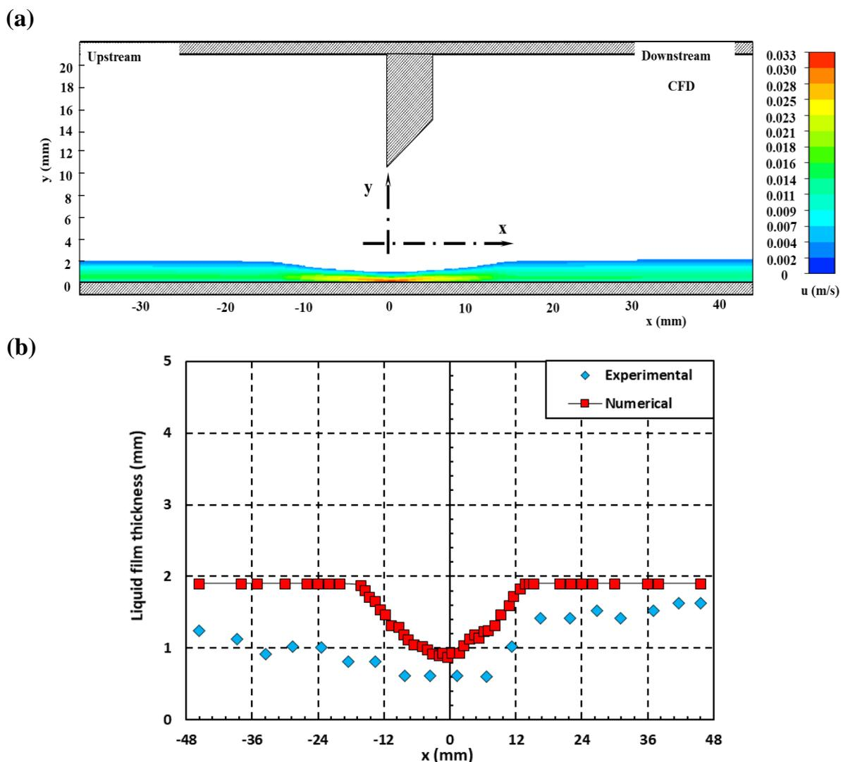
**Figure 48.** Underlying liquid film located at the bottom of the horizontal duct. (a): Averaged axial velocity field. (b): Comparison of experimental (blue diamonds) and numerical simulation (red squares) underlying liquid film thickness. The foam in this simulation was defined by Hershel-Bulkley model.
