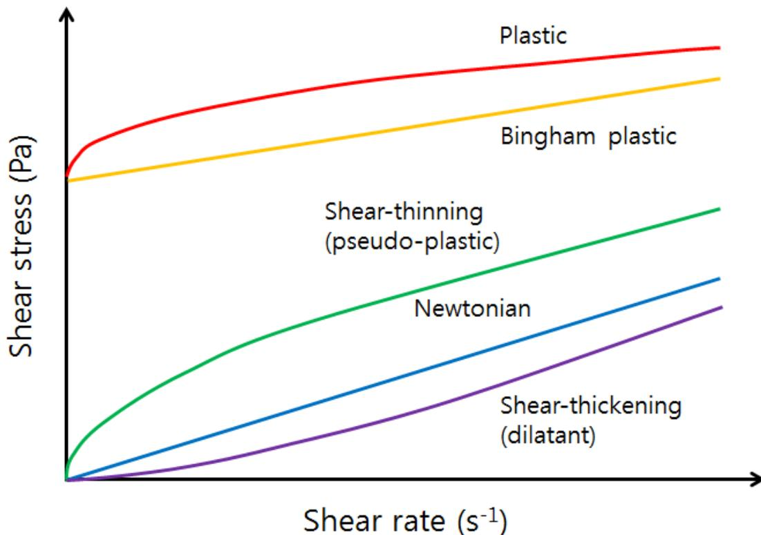
**Figure 14.** Shear in non-Newtonian fluids.
