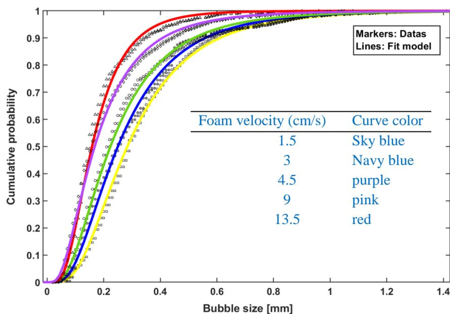
**Figure 63.** Cumulative fraction of the bubble size distribution for all the foam flow conditions. The markers present the brut data and the lines represent the Lognormal model fitted to each condition.
