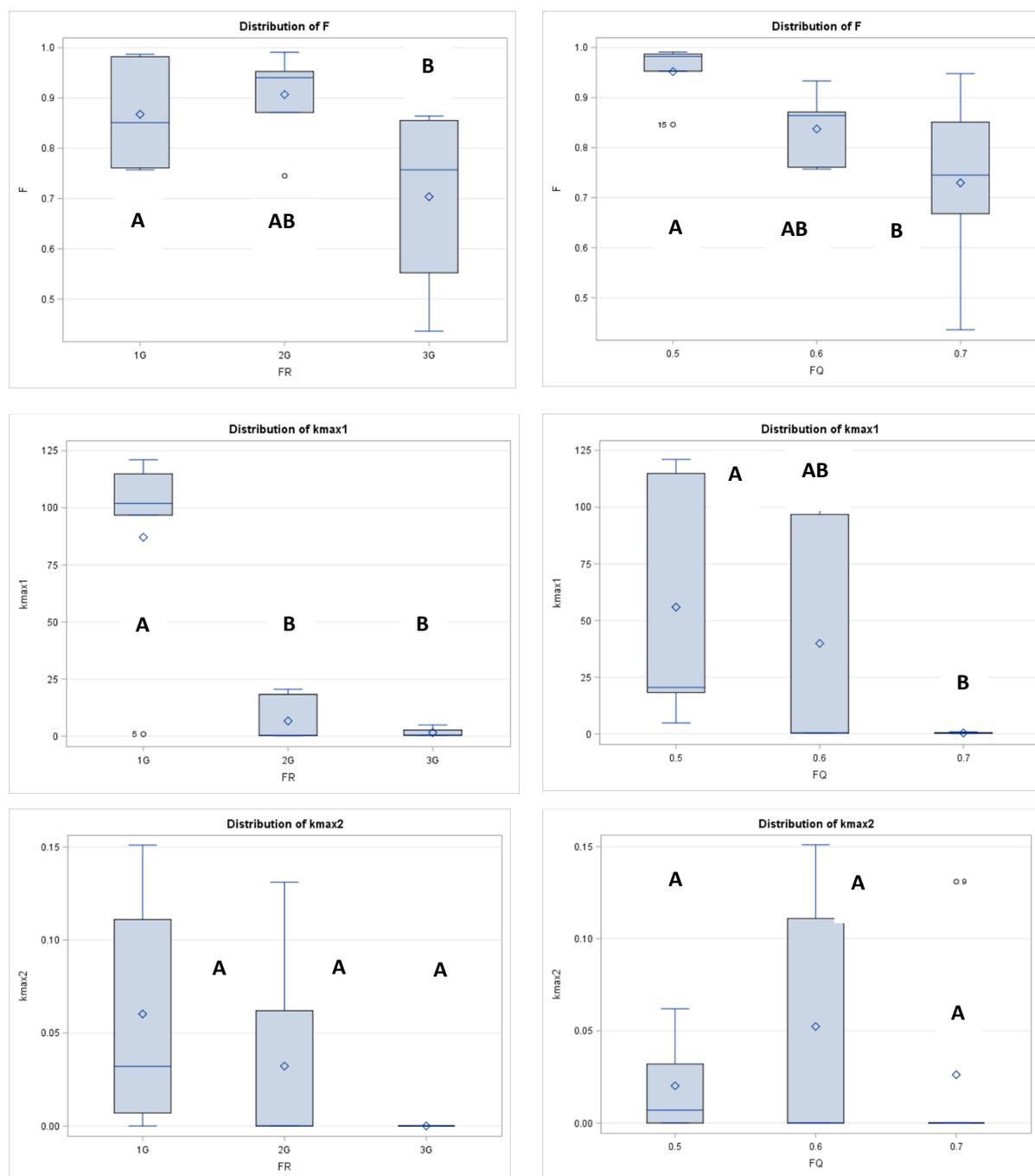
**Figure 57.** Variations induced by the combination of the foam quality (including CIP conditions for the two last graphs) and the flow rate induced by one, two or three generators on the kinetics parameters  $f$ ,  $K_{max1}$  and  $K_{max2}$ . According to the Tukey's grouping letters were indicated with potentially three classes A, AB and B.
