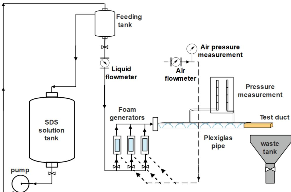
**Figure 51.** Scheme of foam cleaning in place prototype
