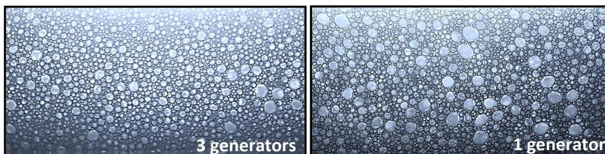
**Supplementary- Figure 72.** Top view of foam visualization at the wall of the transparent pipe upstream the test ducts for foam flow at 9 cm/s, using simultaneously 3 generators (left) or a single generator (right).
