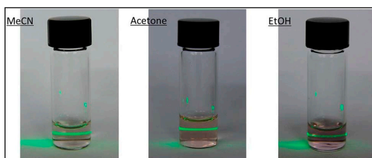
Figure 27. Tyndall effect of crystals of 37 after suspension in acetone, ethanol or acetonitrile (1.0 mg in 1 mL) overnight and then ultrasonicated for 1 min. Reprinted from Reference [172] with permission from The Royal Society of Chemistry.
