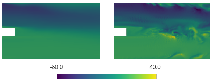
Figure 4.18 – Tangential component of the velocity. On the left: time averaged value. On the right: instantaneous value.
