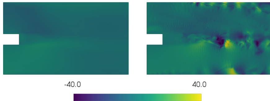
Figure 4.17 – Radial component of the velocity. On the left: time averaged value. On the right: instantaneous value.
