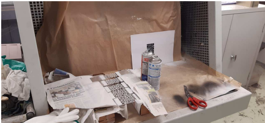
Figure 4.34: Experimental setup for the speckle deposition.
