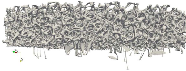
Figure 5.15: Warped reference configuration with the micro displacement solution. Extreme irregular solutions at some finite element nodes are observed.
