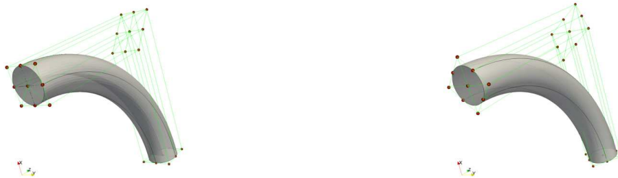
(a) Initial beam geometry obtained from the extrusion of zero radius annulus.
