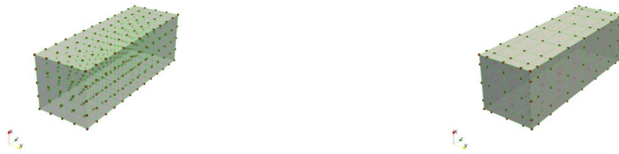
(a) Cuboid discretized with C^0 elements. (b) Cuboid discretized with C^2 elements.
