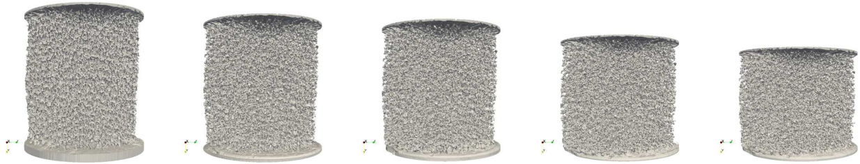
Figure 5.2: Rendering of the reconstructed volumes at the different loading states. The left state is the reference configuration (at rest).
