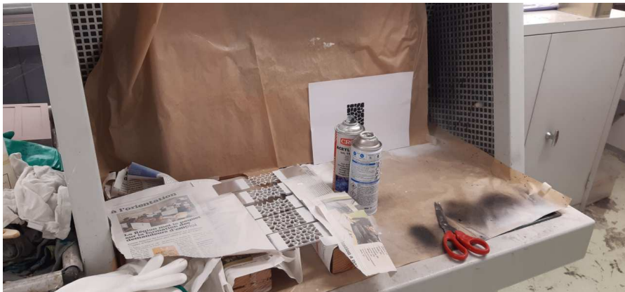
Figure 4.34: Experimental setup for the speckle deposition.
