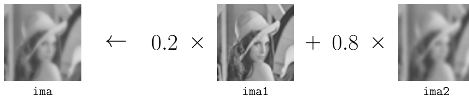
Figure 4.1: Alpha-blending algorithm written at image level.
