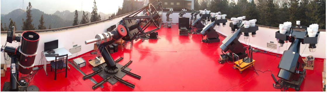
Figure 1.19: View of the GWAC system installed at the Xinglong Observatory in China. On the right part, some of the mounts are visible and on the left part, the 30 and 60 cm telescopes are shown. (SVOM collaboration)
