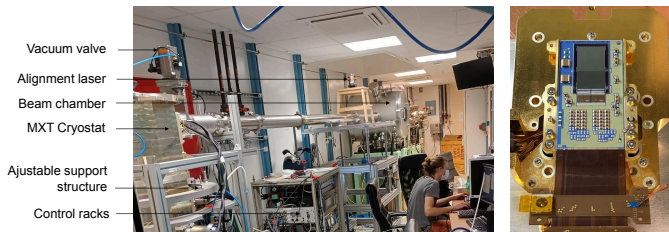
Fig. 2: Test configuration in the experience room. The MXT cryostat is placed 5 meters away from the beam chamber and contains the flight spare model of the focal plane mounted on displacement tables.
