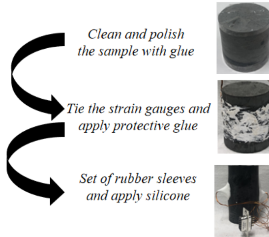
Figure III .2: Steps of attach two pairs of strain gauge to the sample
