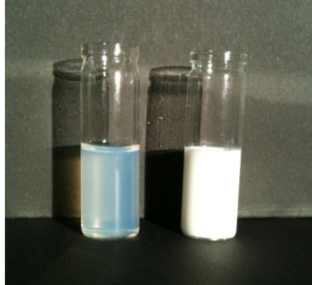
Fig.1. Nano-emulsions with droplet size of 35nm on the left and macro-emulsions with droplet size of 1μm on the right.
