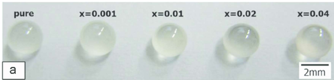
Figure 1.8. Photographs of the as-levitated (Y_{1-x}Eu_x)_3Al_5O_{12} ( x = 0.001, 0.01, 0.02 and 0.04 ) samples; YAG (the first one) and YAG: Eu glass–ceramics with a mass of 38 mg (produced by Chi-Hoon Lee) 18 .
