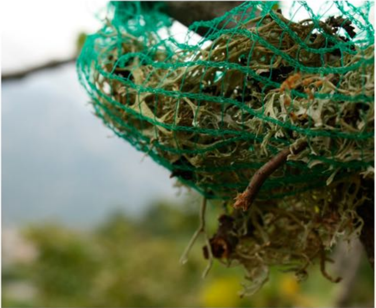
Figure 2.3: Moss bag as a PM bio-sensor in place. Source: Winkler et al. [2020].
