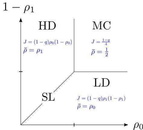
Figure 1.7: Phase diagram of the open ASEP with respect to the boundary parameters (1.47), with the corresponding values of current  $J$  and bulk average density  $\bar{\rho}$ . The phases are: MC maximal current, HD high density, LD low density, SL shock line.
