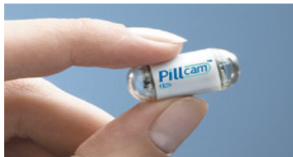
(a) Wireless Capsule Endoscopy device.
