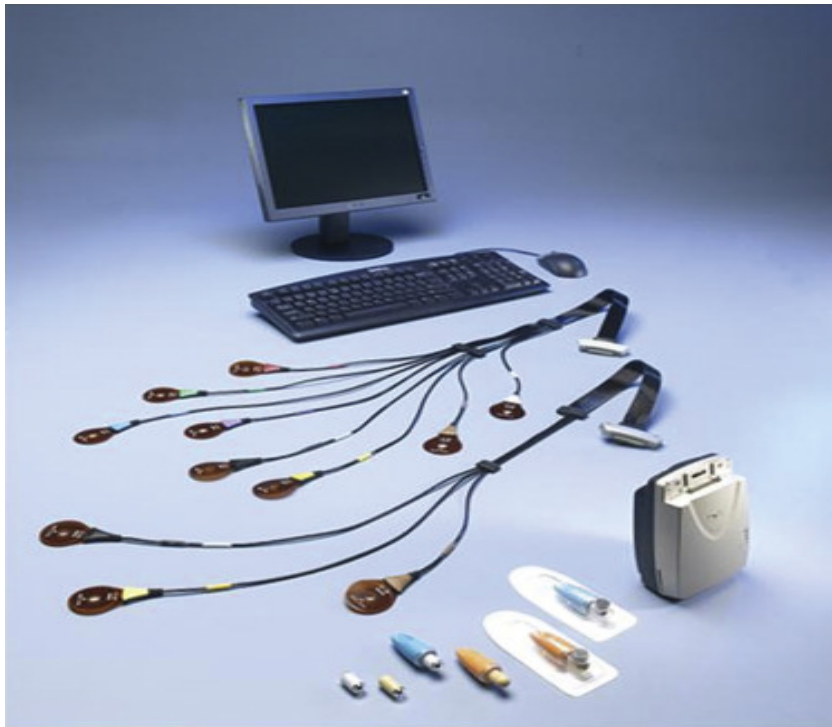
Figure 3.4: The complete system used during a WCE examination. It consists of the capsule device, the sensing system with sensing pads and the data recorder, the battery pack, and the personal computer workstation.
