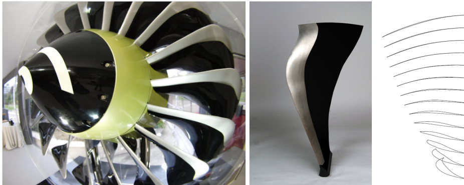
Figure 1: A fan module (left), composed of fan blades (middle) divided into airfoils (right).
