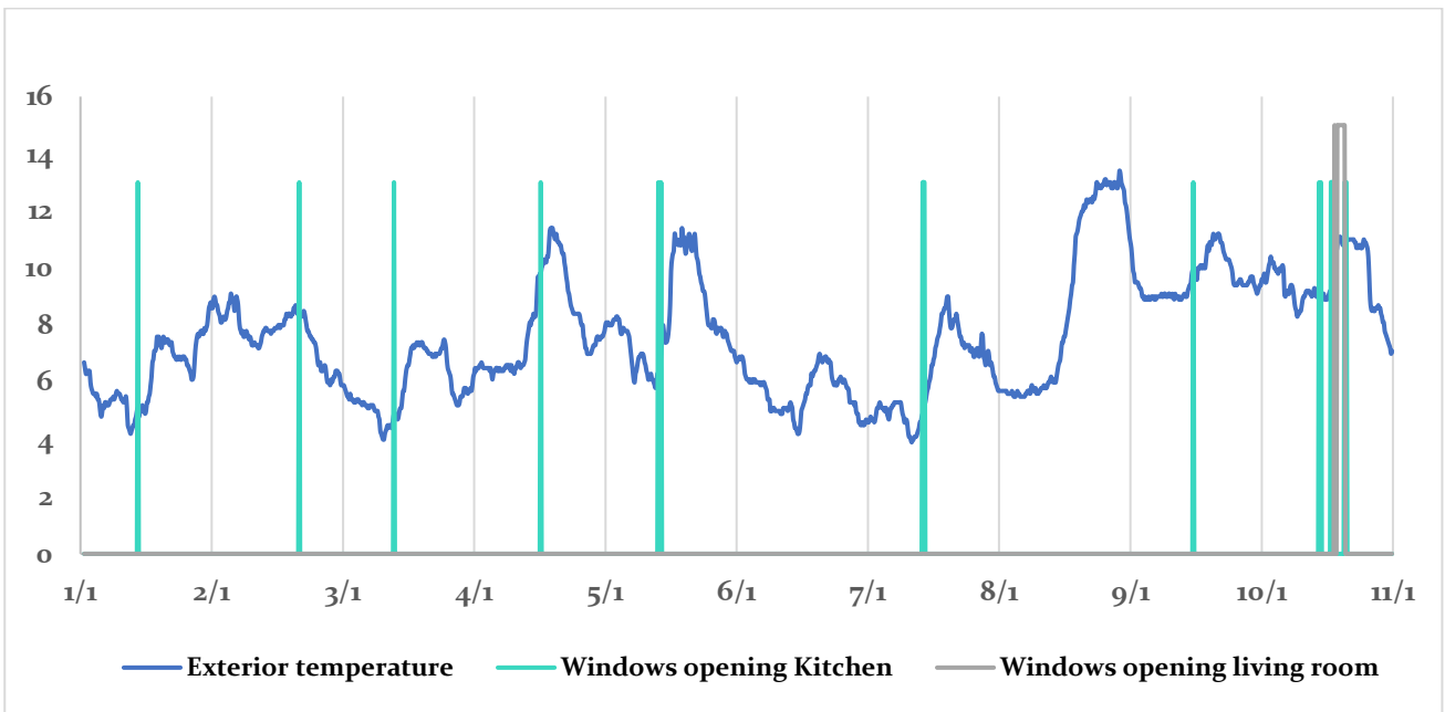
Figure 72: Evolution of the outdoor temperature according to windows opening in Kitchen and Stay (from 01/01 to 10/01).
