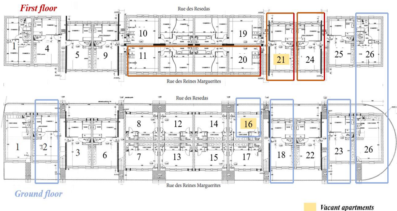
Figure 14: The plan of the building and the selection of the dwellings for instrumentation.
