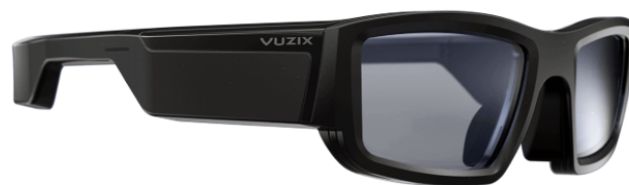
Fig. 4.7 AR glasses used for this study (Vuzix Blade AR Smart Glasses)
