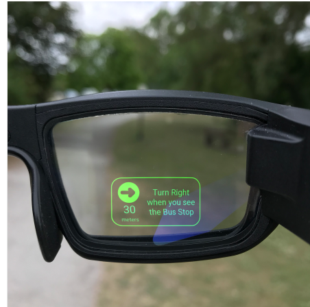
Fig. 5.6 AR Glasses Application displaying the instruction: "Turn Right when you see the Bus Stop in 30 meters"
