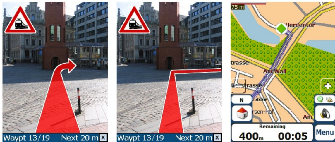
Fig. 2.4 Screenshots of the prototype interface with arrow and line visualisation; The Destination 6 interface with a 2D map in pedestrian mode [111]
