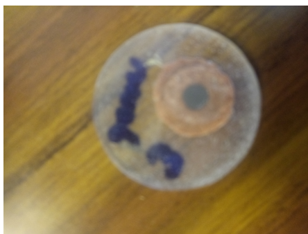
Figure 5.3: The gasket embedded in the resin and then polished, in order to facilitate Raman spectroscopy. The sample was polished on both the top and bottom circular surfaces and one of these sides is shown in the image. The black circle seen in the centre of the gasket is the sample. Raman spectroscopy was done in various points on the sample surface.
