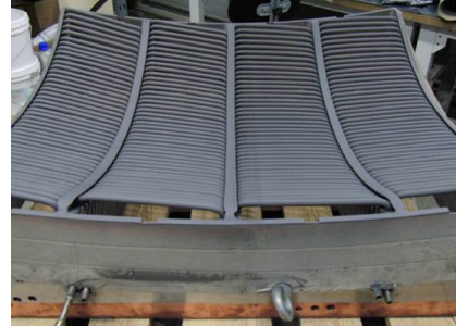
Faraday screen with B_4C layer [3]
