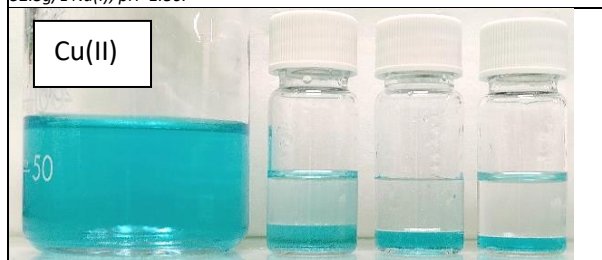
Figure 48. From the left to the right: Stock solution Cu(II) in \text{Na}_2\text{SO}_4/\text{H}_2\text{O} ; biphasic samples: 20/80, 30/70, 40/60 wt% of PEG-400/stock solution. The stock solution is made by 5g/L of Cu(II), from \text{CuSO}_4 \cdot 5\text{H}_2\text{O} salt, 105g/L of \text{SO}_4^{2-} , 45g/L Na(I), pH=1.87.
