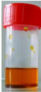
Figure 72. Sample prepared to demonstrate the PEG-400 extraction efficiency on the \text{Na}_2\text{SO}_4 bath. Repartition used 50/50 wt% of polymer/bath.
