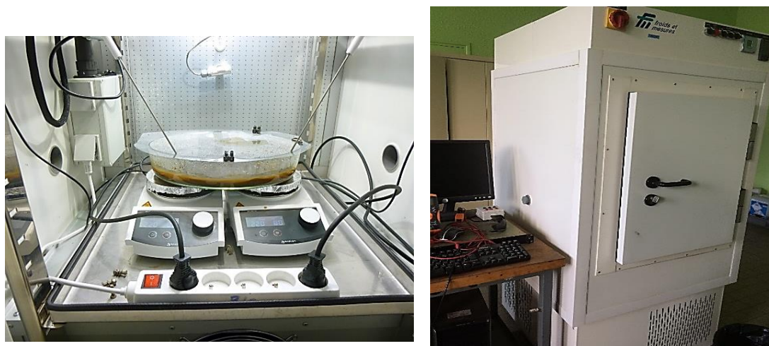
Figure 108. Light box used as UV source for step 2.
