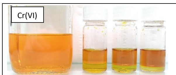
Figure 46. From the left to the right: Stock solution Cr(VI) in \text{Na}_2\text{SO}_4/\text{H}_2\text{O} ; biphasic samples: 20/80, 30/70, 40/60 wt% of PEG-400/stock solution. The stock solution is made by 5g/L of Cr(VI), from \text{Na}_2\text{Cr}_2\text{O}_7 \cdot 2\text{H}_2\text{O} salt, 105g/L of \text{SO}_4^{2-} , 52.3g/L Na(I), pH=1.80.
