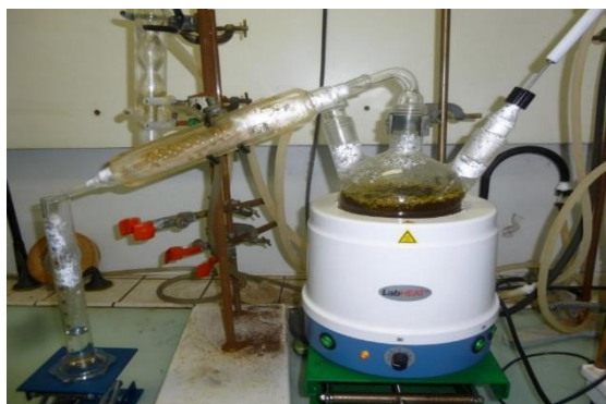
Figure 121. Step 3 - Distillation process proposed in this work (700g of polymer treated).
