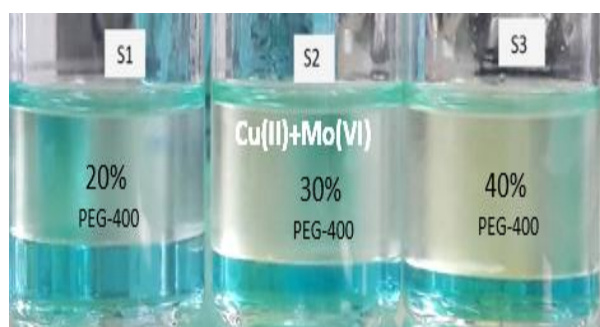
Figure 86. Samples obtained by mixing different wt% of PEG-400 + stock solution Cu(II)+Mo(VI); s1 = 20/80, s2 = 30/70, s3 = 40/60, in wt%, of PEG-400/stock solution.
