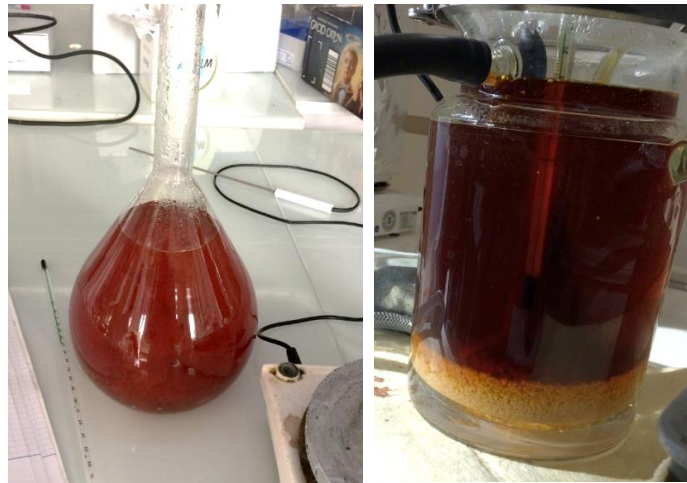
Figure 94. On the left - formation of crystal structures in the \text{Na}_2\text{SO}_4 bath with a temperature superior of 50^\circ\text{C} . On the right - solid precipitation occurred during the continuous process.
