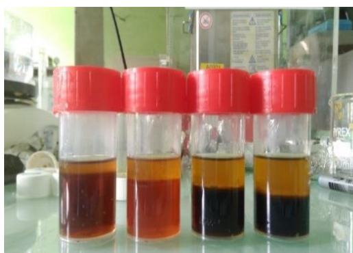
Figure 71. Samples prepared for demonstrating the PPG-425 extraction efficiency on the \text{Na}_2\text{SO}_4 bath. Starting from the left to the right: 10/90-20/80-30/70-40/60 wt% of PPG-425/ \text{Na}_2\text{SO}_4 bath.
