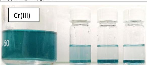
Figure 49. From the left to the right: Stock solution Cr(III) in  $\text{Na}_2\text{SO}_4/\text{H}_2\text{O}$ ; biphasic samples: 20/80, 30/70, 40/60 wt% of PEG-400/stock solution. The stock solution is composed by 0.62 g/L of Cr(III), from  $\text{Cr}_2(\text{SO}_4)_3$  anhy. salt, 93 g/L of  $\text{SO}_4^{2-}$ , 43.63 g/L Na(I), pH=1.77
