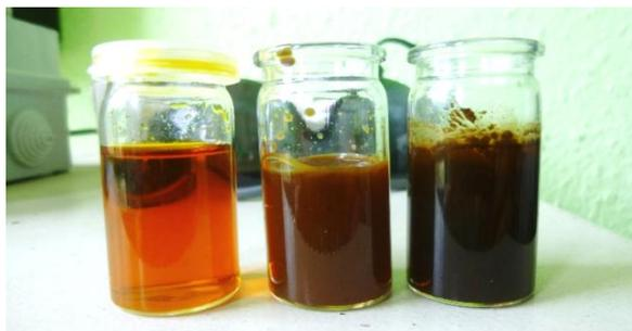
Figure 106. UPS1 exposed to the sunlight. Starting from the left to the right: UPS1 as soon as was separated from the lower phase in the step 1, UPS1 exposed to the sunlight for 12 hours, UPS1 exposed to the sunlight for 24 hours.
