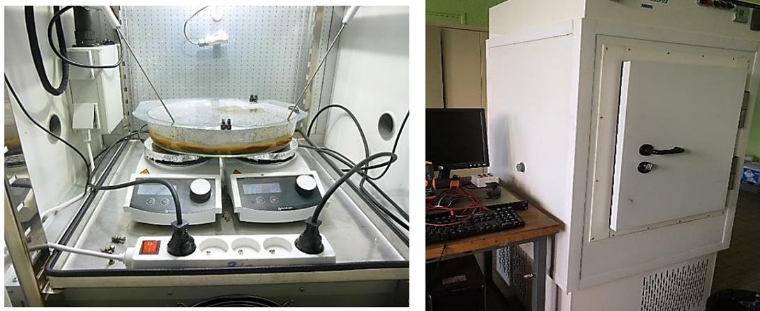
Figure 108. Light box used as UV source for step 2.
