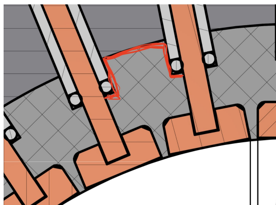
Figure 5.17. – Leaking current inside the EIT sensor due to the apparition of a gap (in red) between the electrodes.
