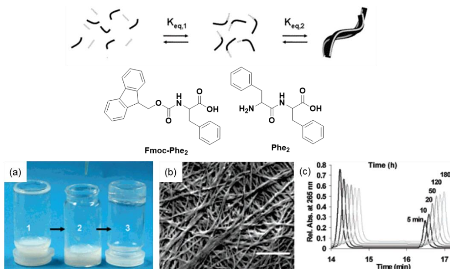
Figure 1.33 | Enzyme-triggered self-assembly of peptide hydrogels via reversed hydrolysis. a) 1: Suspension of Fmoc-Phe and (Phe)_2 . 2: addition of 0.5 mg of thermolysin. 3: Inversion demonstrates self-supporting gel formation; b) Cryo-SEM micrograph of enzymatically prepared Fmoc- (Phe)_3 hydrogel obtained from 40 \mu mol of Fmoc-Phe and (Phe)_2 and 0.5 mg thermolysin. The scale bar represents 0.5 \mu m. c) HPLC chromatograms of peptide synthesis in the course of time in the presence of 0.5 mg thermolysin. Peaks shown represent Fmoc-Phe and Fmoc- (Phe)_3 . Figure is reproduced and adapted from ref. 104 .
