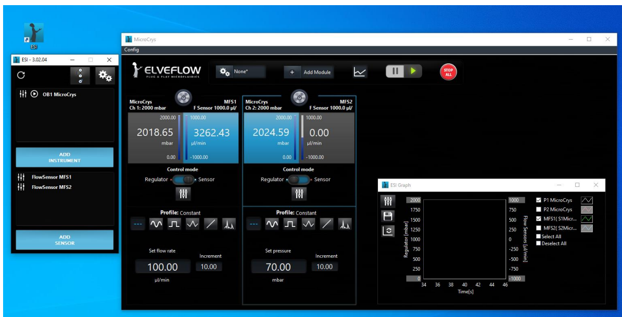
Figure 3.2.10: The ESI (Elveflow Smart Interface) software illustrating the two pressure channels used for the on chip crystallization experiments conducted with the MicroCrys platform.
