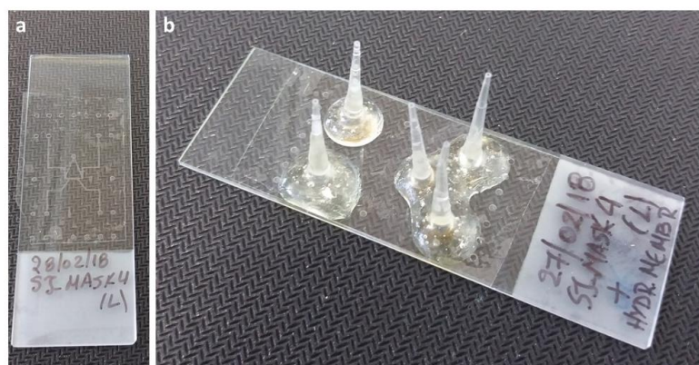
Figure 2.3.6: (a) PEGDA chip fabricated directly from the SU-8 master and (b) the pipette tips used as connectors on the inlet and outlet ports.
